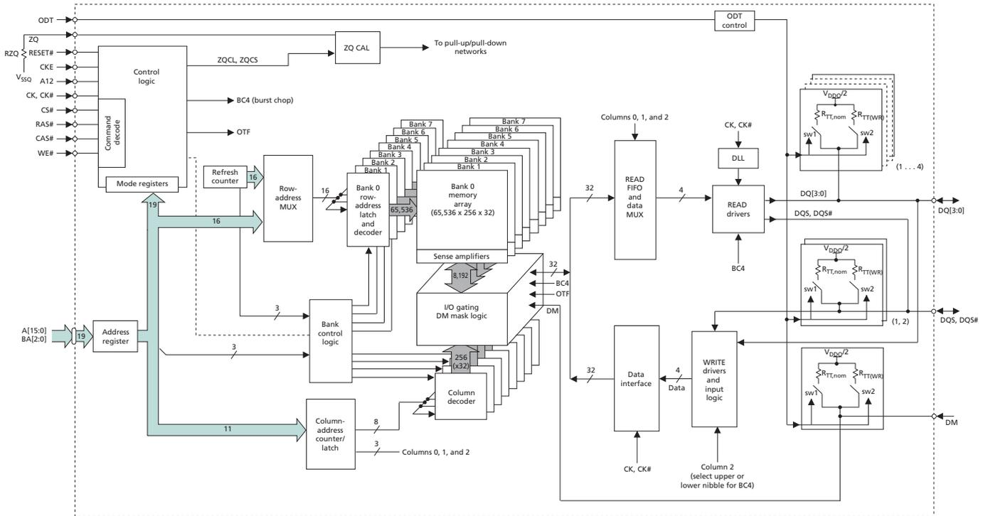
**Figure 4: 512 Meg x 8 Functional Block Diagram**
