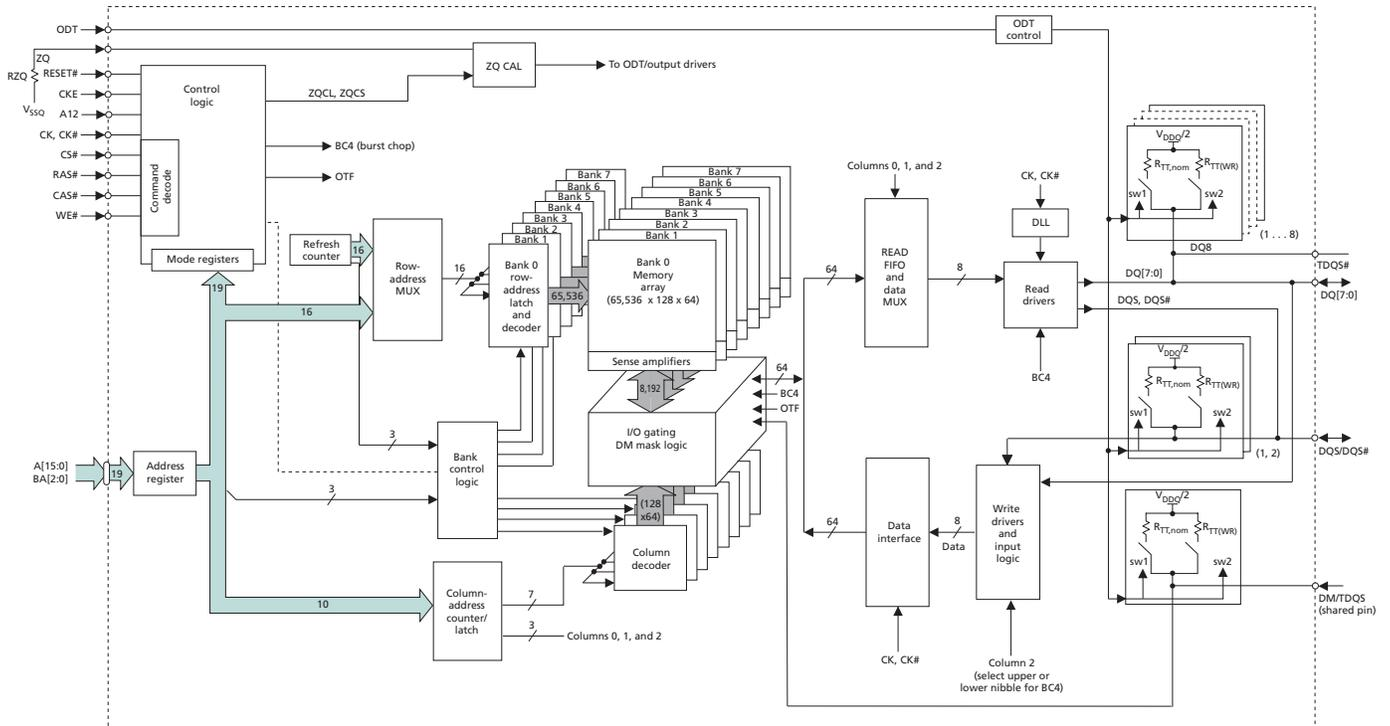
**Figure 5: 256 Meg x 16 Functional Block Diagram**
