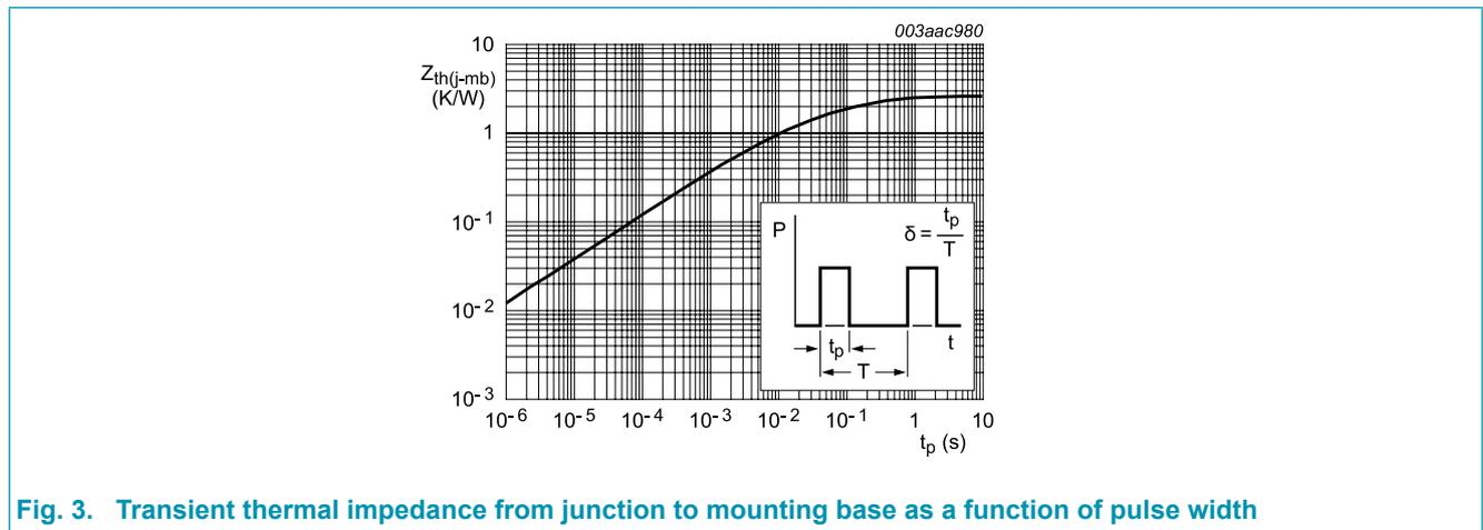
Fig. 3. Transient thermal impedance from junction to mounting base as a function of pulse width
