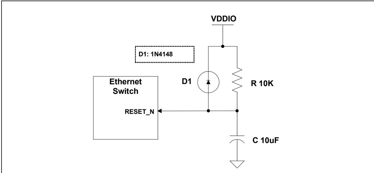
Figure 7-2 illustrates a reset circuit recommended for applications where reset is driven by another device, such as a CPU. At power-on reset, R, C and D1 provide the necessary ramp rise time to reset the KSZ9893R. The RST\_OUT\_N from the CPU provides a warm reset after power-up.
