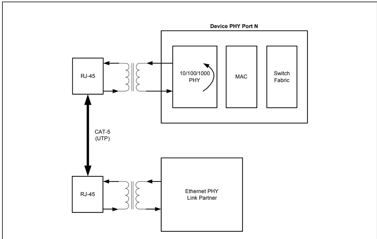
The following programming steps and register settings are for remote PHY loopback mode for 1000BASE-T Master Mode, 1000BASE-T Slave Mode, 100BASE-TX Mode, and 10BASE-T Mode.
