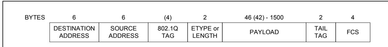
When the switch forwards a received packet to the host port, one tail tagging byte is added to the packet by the switch to indicate to the host processor which port the packet was received on. The format is shown in [Table 4-13](#).
