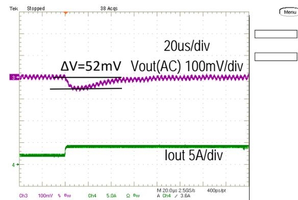
Step Load Transient Response (Vin=12V, Vout=5.0V, Cloud=400uF, Iout=4A to 2A, 2.5A/us)
