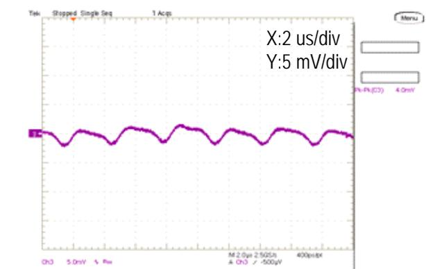
Step Load Transient Response (Vin=12V, Vout=1.0V, Cloud=400uF, Iout=2A to 4A, 2.5A/us)
