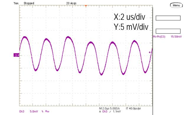
Step Load Transient Response (Vin=12V, Vout=5.0V, Cloud=400uF, Iout=2A to 4A, 2.5A/us)
