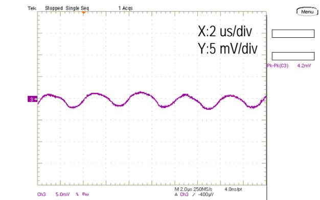
Step Load Transient Response (Vin=5.0V, Vout=1.8V, Cload=400uF, Iout=2A to 4A, 2.5A/us)
