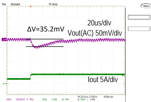
Step Load Transient Response (Vin=12V, Vout=3.3V, Clod=400uF, Iout=4A to 2A, 2.5A/us)
