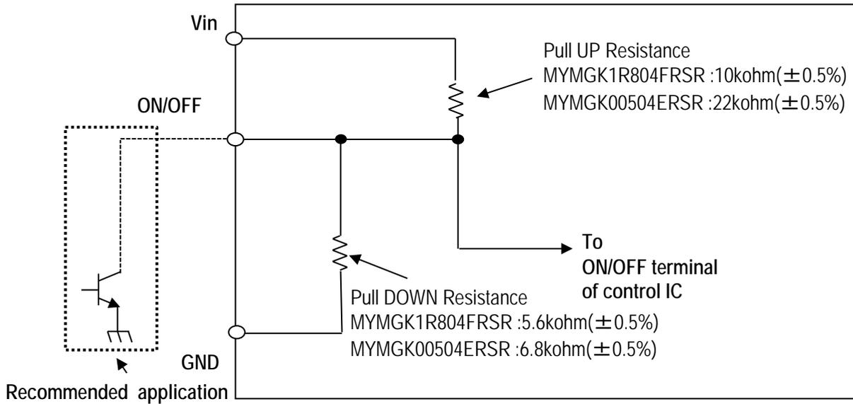
PowerGood(P.G) internal circuit diagram and using guide
