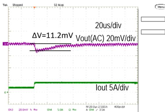
Step Load Transient Response (Vin=12V, Vout=1.0V, Cloud=400uF, Iout=4A to 2A, 2.5A/us)
