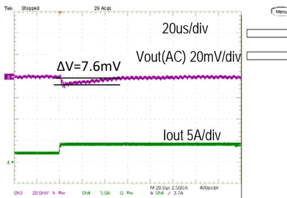
Step Load Transient Response (Vin=5.0V, Vout=0.7V, Cload=400uF, Iout=4A to 2A, 2.5A/us)
