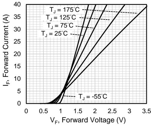
Fig.1 Forward Characteristics
