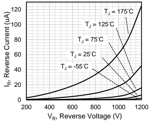
Fig.2 Reverse Characteristics
