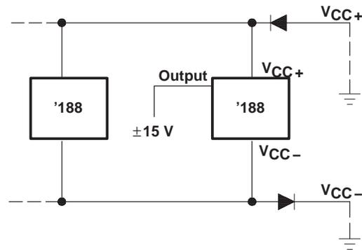
Diodes placed in series with the  $V_{CC+}$  and  $V_{CC-}$  leads protect the SN55188/SN75188 in the fault condition in which the device outputs are shorted to  $\pm 15 \text{ V}$ , and the power supplies are at low voltage and provide low-impedance paths to ground.
