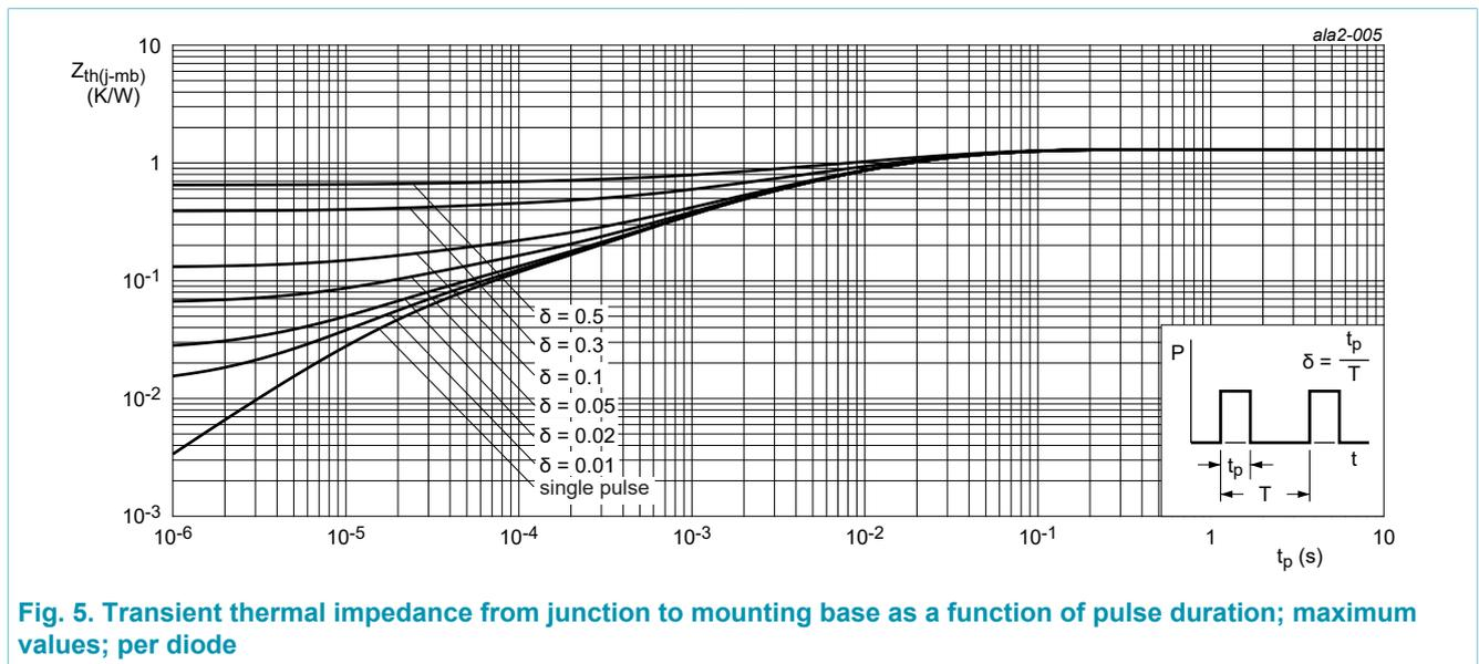
Fig. 5. Transient thermal impedance from junction to mounting base as a function of pulse duration; maximum values; per diode
