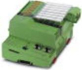
Inline controller with integrated pulse/direction/PWM interface, RS-485/RS-422, analog inputs (0 ... 10 V), and analog outputs (0 ... 10 V), with programming options according to IEC 61131-3
