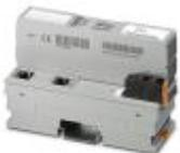
Axiocontrol for the direct control of Axiline I/Os. With 2 Ethernet interfaces, extended temperature range, and programming options according to IEC 61131-3. Complete with connector connector and marking field.
