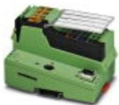
The Inline controller offers the option of communicating via PROFINET and Modbus/TCP. Programming is carried out using PC Worx Express or PC Worx (IEC 61131-3).
