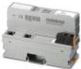
Axio control for direct open-loop control of Axiline I/Os. With 2 Ethernet interfaces and programming capabilities according to IEC 61131-3. Complete with connector connector and labeling field.
