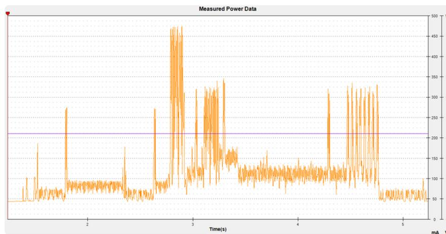
You can put the FONA into sleep mode (with the `AT+CSCCLK` command) which will drop the current draw but keep the cellular connection open so you can still receive an SMS and/or wakeup quickly.
