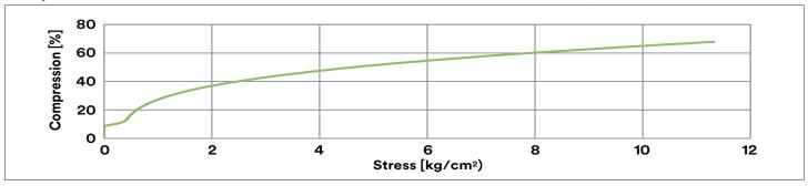
Sample size: 1.0T, 30 by 30mm Test speed: 0.5mm/min
