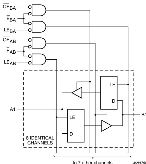
Fig.5 Logic diagram.
