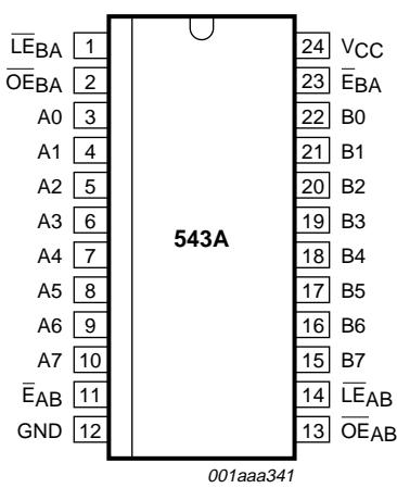
Fig.1 Pin configuration SO24 and (T)SSOP24.
