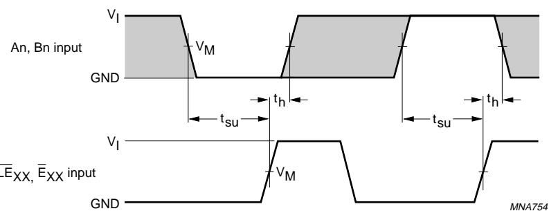
$$V_M = 1.5 \text{ V at } V_{CC} \geq 2.7 \text{ V.}$$
