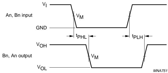
$V_M = 1.5 \text{ V}$  at  $V_{CC} \geq 2.7 \text{ V}$ . $V_M = 0.5 \times V_{CC}$  at  $V_{CC} < 2.7 \text{ V}$ . $V_{OL}$  and  $V_{OH}$  are typical output voltage drop that occur with the output load.
