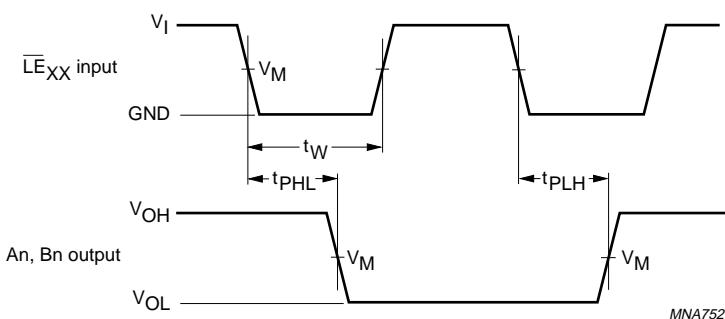
$V_M = 1.5 \text{ V}$  at  $V_{CC} \geq 2.7 \text{ V}$ . $V_M = 0.5 \times V_{CC}$  at  $V_{CC} < 2.7 \text{ V}$ . $V_{OL}$  and  $V_{OH}$  are typical output voltage drop that occur with the output load.Fig.7 Latch enable input ( $\overline{LE}_{XX}$ ) pulse width and latch enable input to output An and Bn propagation delays.
