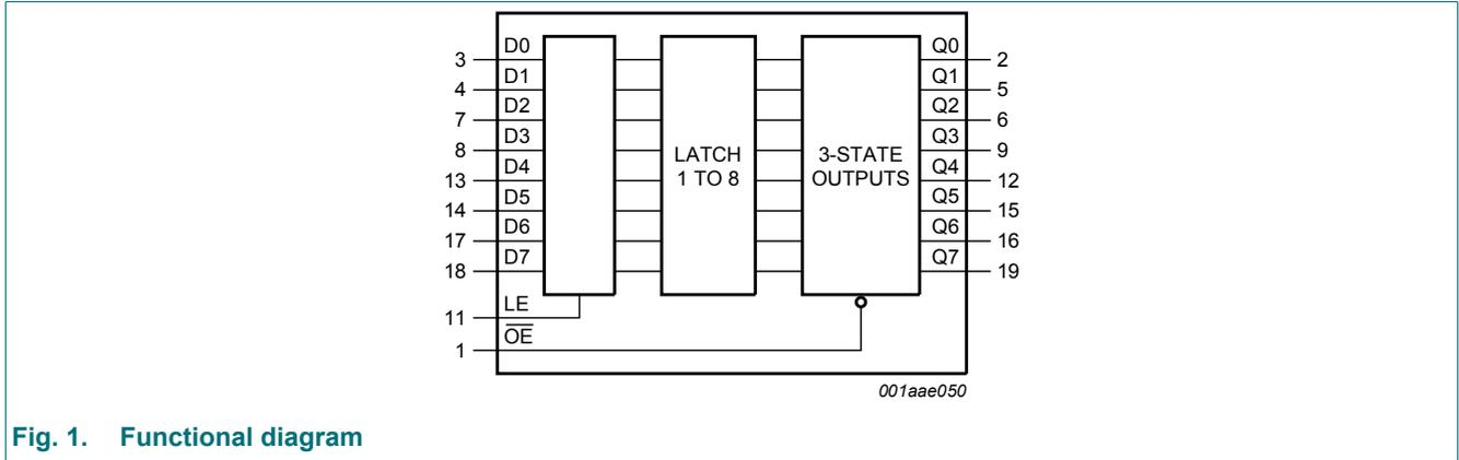
Fig. 1. Functional diagram
