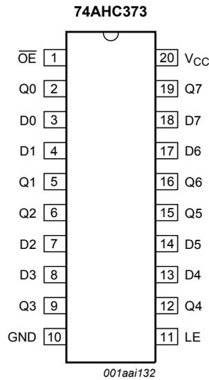
Fig. 6. Pin configuration SOT163-1 (SO20) and SOT360-1 (TSSOP20)
