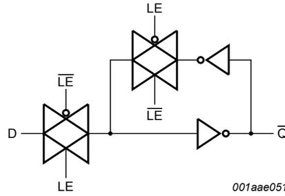
Fig. 5. Logic diagram (one latch)
