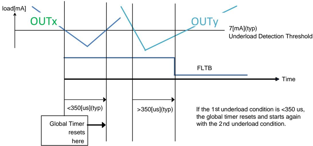
**Figure 9. Underload Discontinuous Time**
