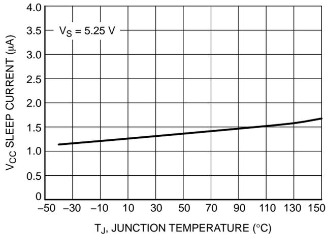
Figure 4. V<sub>CC</sub> Sleep Supply Current vs. Temperature
