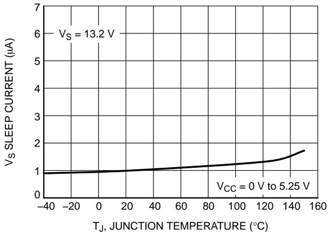
Figure 3. V<sub>S</sub> Sleep Supply Current vs. Temperature
