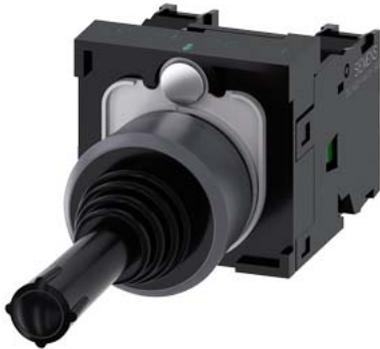
Coordinate switch, 22 mm, round, plastic with metal front ring, black, 2 switch positions, horizontal, momentary contact type, without mechanical interlocking in O position, with holder, 1 NO, 1 NO, screw terminal, with laser labeling, upper case
