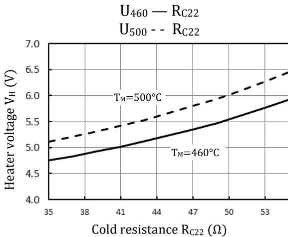
Mean<sup>1</sup> and upper bound of heater voltage V<sub>H</sub> vs. cold resistance R<sub>C22</sub>
