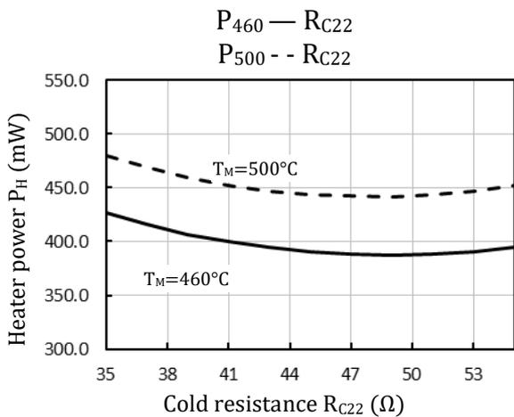
Mean<sup>1</sup> and upper bound of heater power P<sub>H</sub> vs. cold resistance R<sub>C22</sub>
