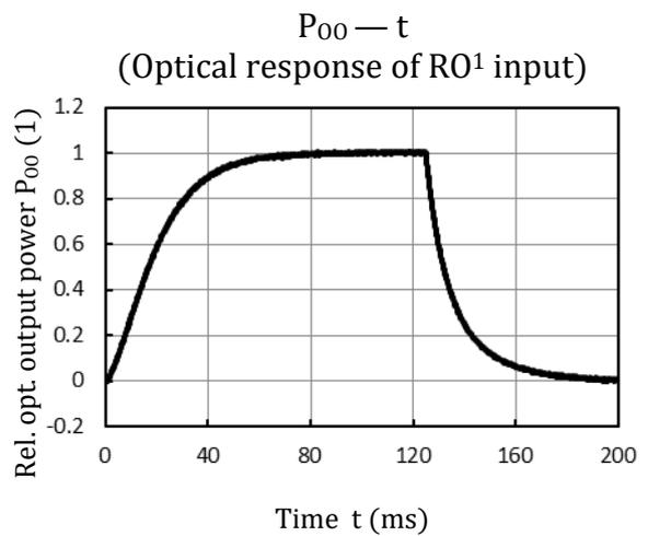
Optical response time (relative optical output power P<sub>00</sub>) of a rectangular voltage pulse (RO<sup>1</sup> conditions)
