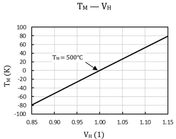
Relative change of membrane temperature (T<sub>M</sub>) by changing heater voltage (V<sub>H</sub>)
