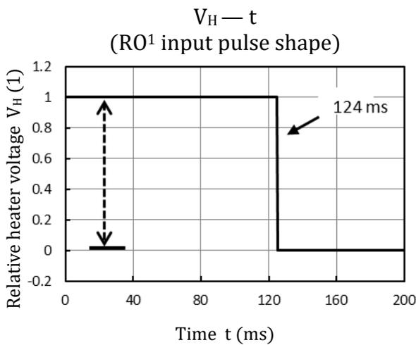
Relative rectangular heater voltage (V<sub>H</sub>) pulse with a relative pulse width of 124 ms at 5 Hz (time description of reference operation RO<sup>1</sup>)
