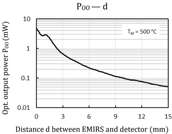
Optical output power ( $P_{00}$ ) versus distance  $d$  of a 1 mm<sup>2</sup> detection surface at 500°C  $T_M$
