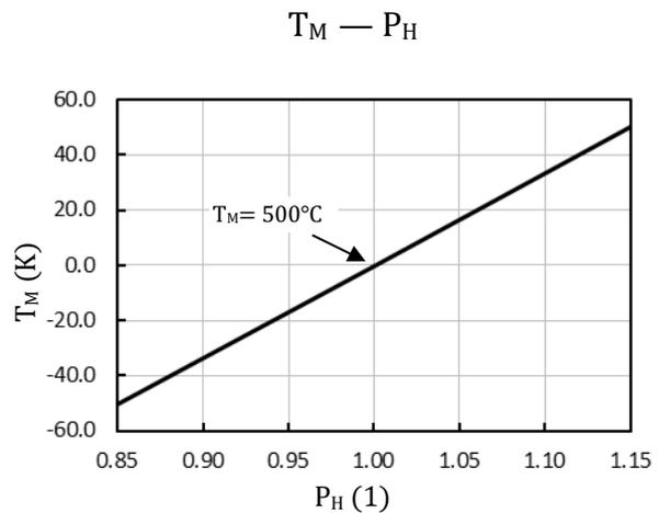
Relative change membrane temperature (T<sub>M</sub>) by changing heater power (P<sub>H</sub>)
