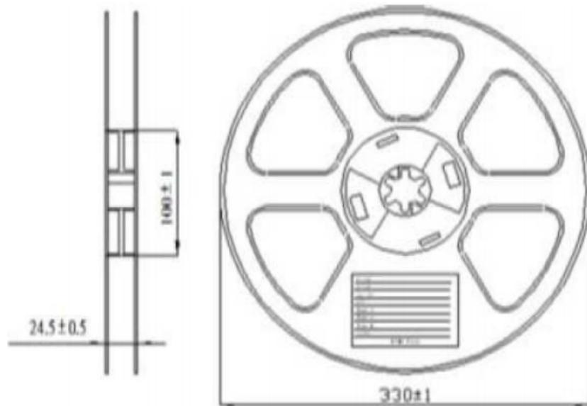
Dimension of Tape (Unit: mm)
