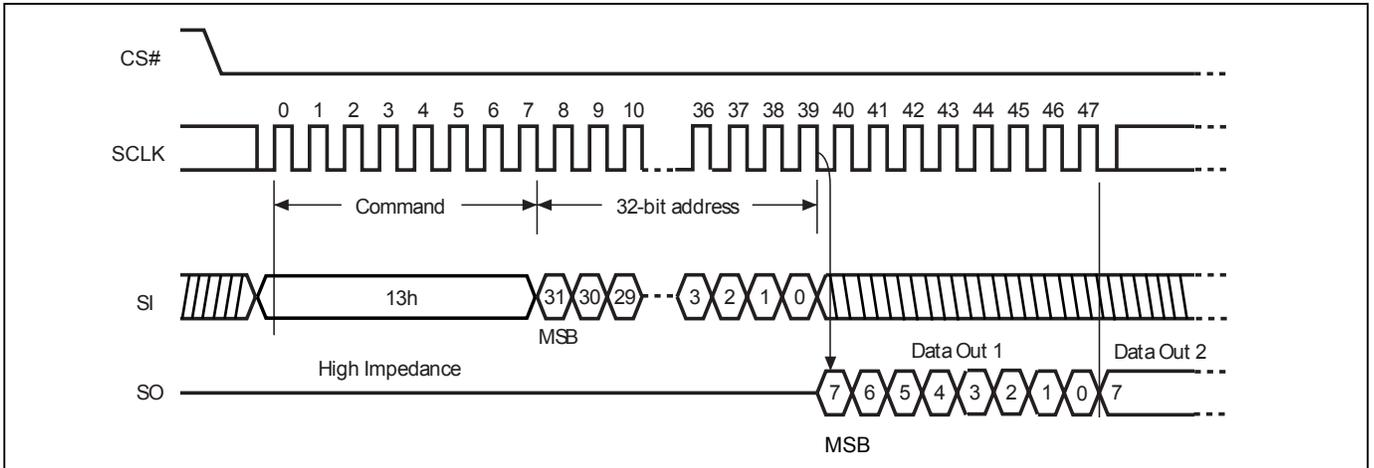
**Figure 47. Read Data Bytes at Higher Speed using 4 Byte Address Sequence (FASTREAD4B)**
