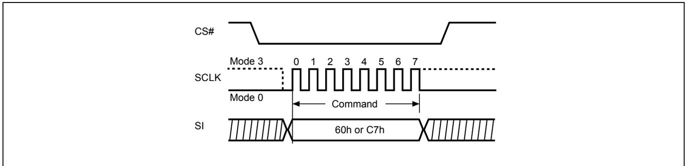
**Figure 63. Chip Erase (CE) Sequence (QPI Mode)**
