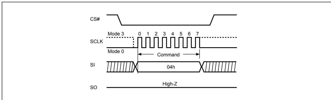
**Figure 12. Write Disable (WRDI) Sequence (QPI Mode)**
