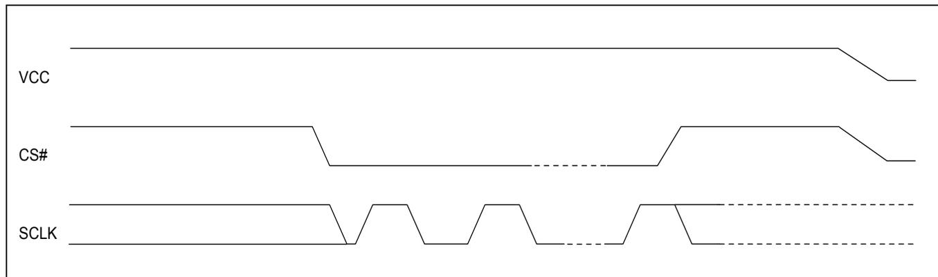
**Figure 97. Power-up Timing**
