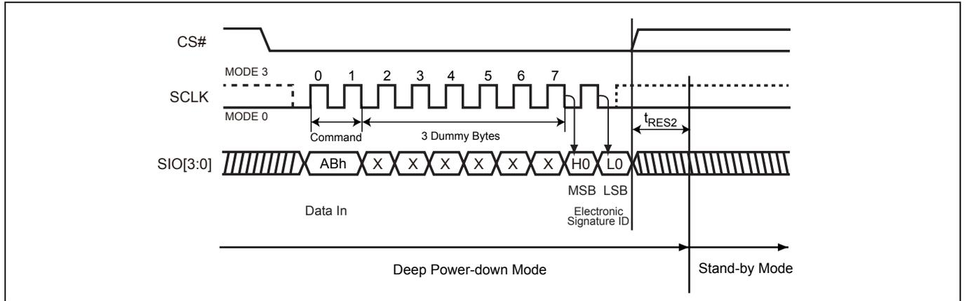
**Figure 18. Release from Deep Power-down (RDP) Sequence (SPI Mode)**
