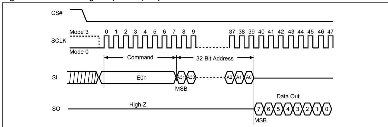
**Figure 81. Write DPB Register (WRDPB) Sequence**
