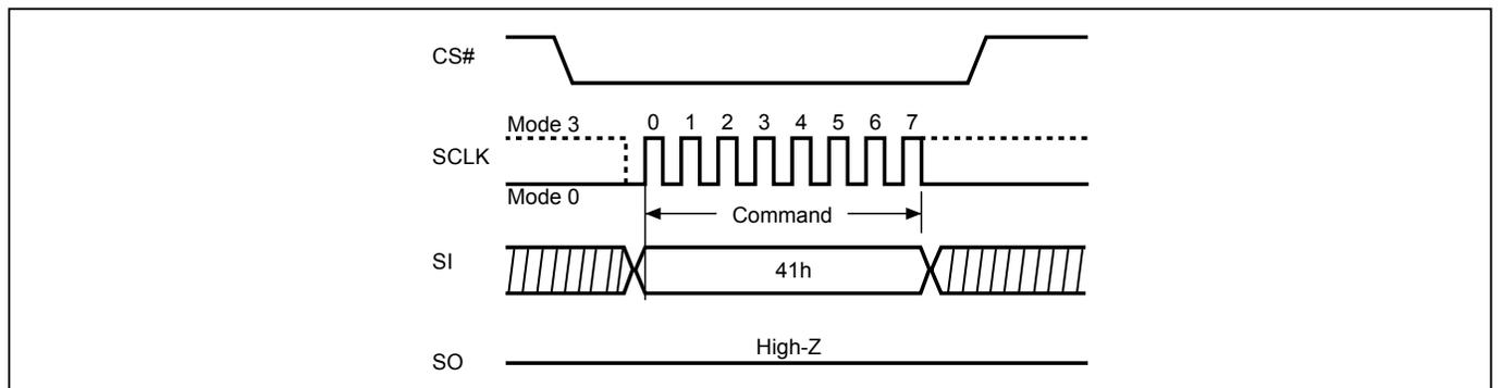
**Figure 14. Factory Mode Enable (FMEN) Sequence (QPI Mode)**
