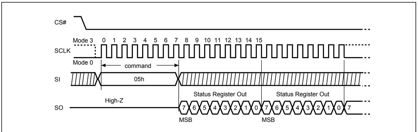
**Figure 22. Read Status Register (RDSR) Sequence (QPI Mode)**
