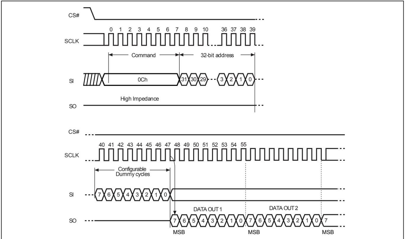
**Notes:** Configuration Dummy cycle numbers will be different depending on the bit6 & bit7 (DC0 & DC1) setting in configuration register.
