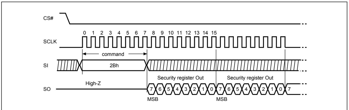
**Figure 72. Read Security Register (RDSCUR) Sequence (QPI Mode)**
