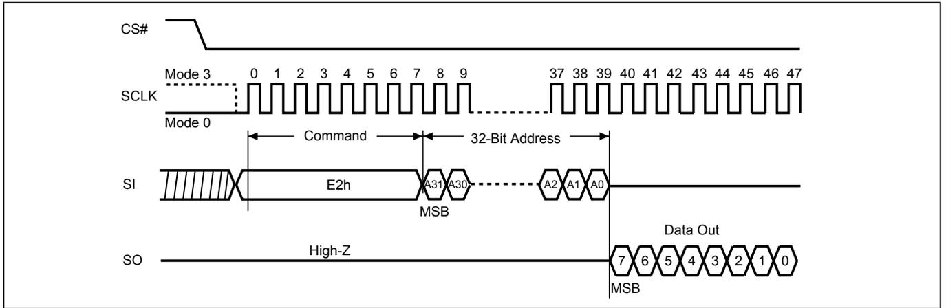
**Figure 78. SPB Erase (ESSPB) Sequence**
