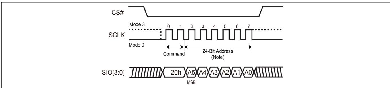
**Note:** Please note the address cycles above are based on 3-byte address mode. For 4-byte address mode, the address cycles will be increased.
