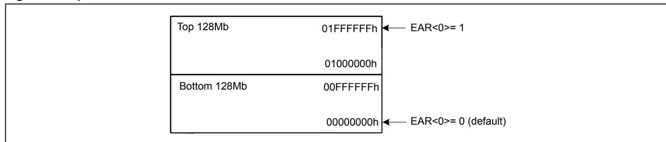
When under EAR mode, Read, Program, Erase operates in the selected segment by using 3-byte address mode.
