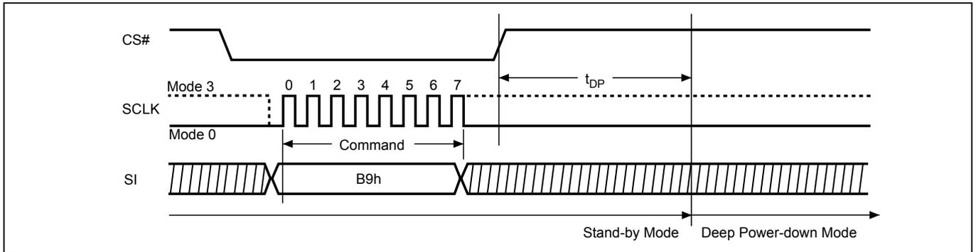
**Figure 68. Deep Power-down (DP) Sequence (QPI Mode)**
