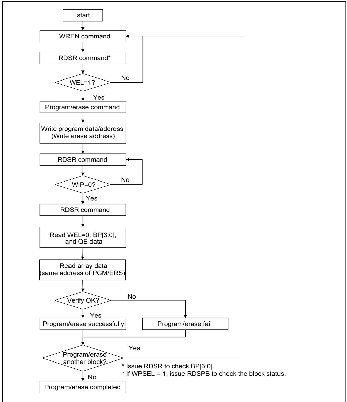
Figure 26. Program/Erase flow without read array data (read P\_FAIL/E\_FAIL flag)
