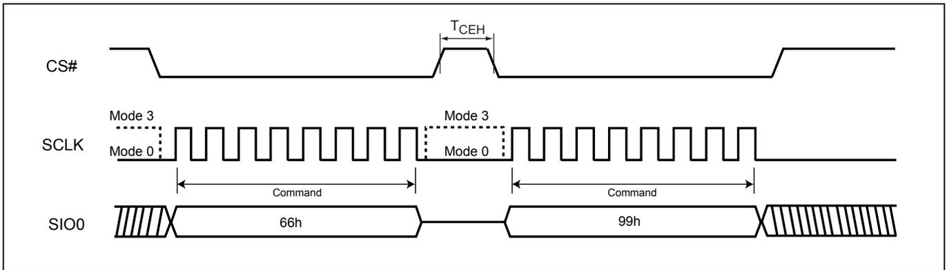
**Figure 87. Reset Sequence (QPI mode)**
