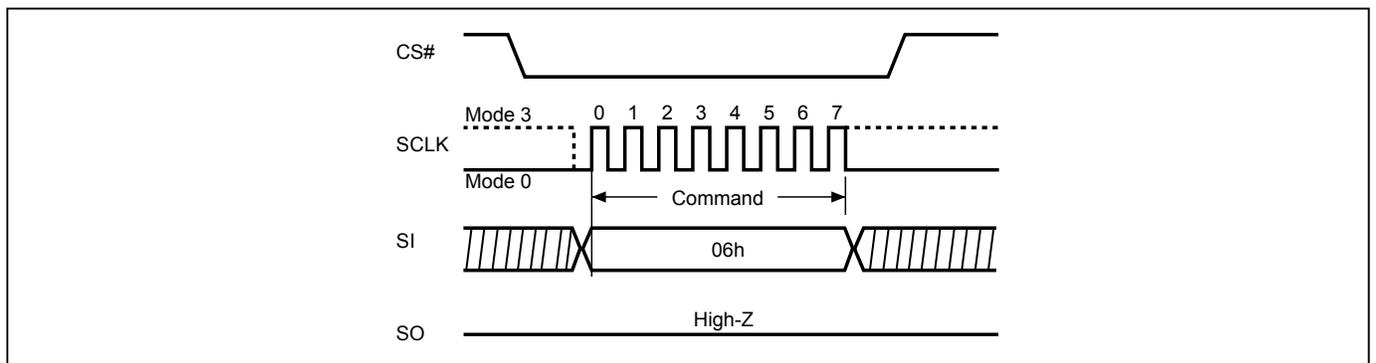
**Figure 10. Write Enable (WREN) Sequence (QPI Mode)**
