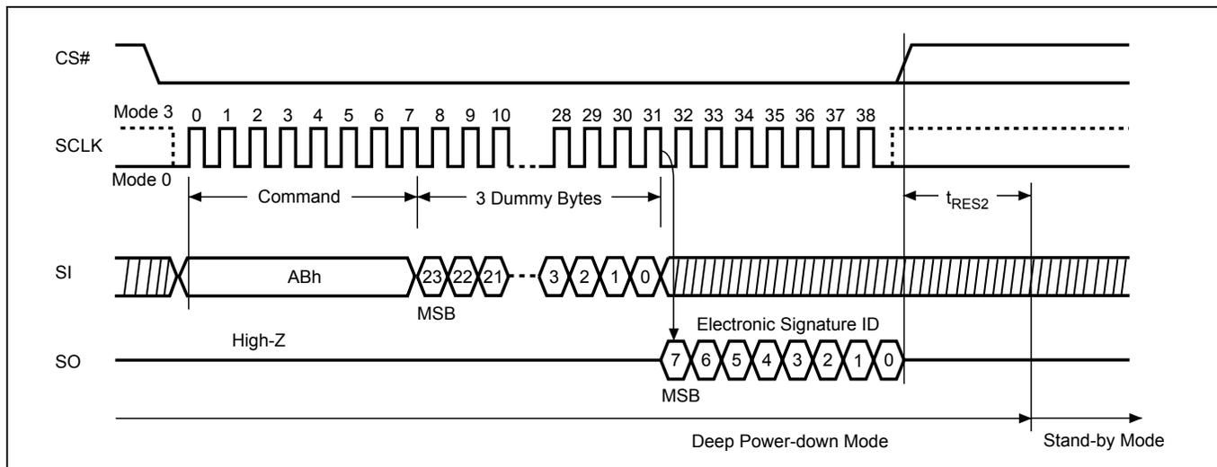
**Figure 17. Read Electronic Signature (RES) Sequence (QPI Mode)**
