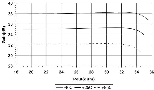
Typical Gain vs Pout, F=3.6GHz
