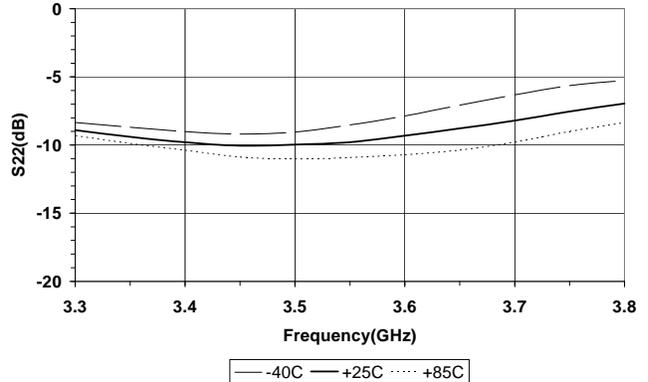
Measured 3.3GHz to 3.6GHz Application Circuit Data ( $V_{CC}=V_{PC}=5.2V$ ,  $I_Q=800mA$ ,  $T=25^\circ C$ )
