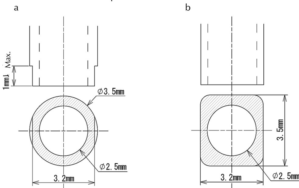
Nozzle with chamfering is recommended
