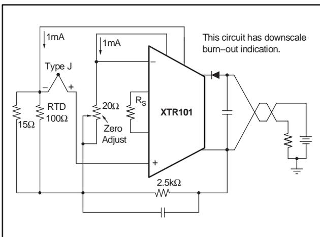
Figure 16. Thermocouple Input with RTD Cold Junction Compensation
