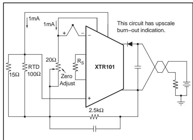
Figure 18. Thermocouple Input with RTD Cold Junction Compensation
