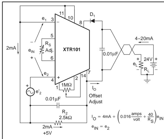
**Figure 5. Basic Connection for Floating Voltage Source**
