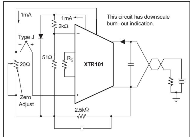
Figure 17. Thermocouple Input with Diode Cold Junction Compensation
