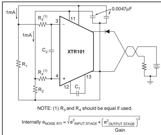
**Figure 12. Optional Filtering**
