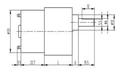
•Rated Voltage: DC 12V •No load speed: 319rpm •No Load Current: 100mA •load torque: 0.28kg.cm •load Speed: 255rpm •load Current: 170mA •load out put: 0.8w •Stall torque: 1.1kg.cm •Stall Current: 1.2kg.cm
