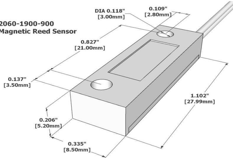
All measurements are in Inches [millimeters]
