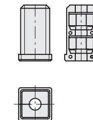
The geometry of the end-cap in the part that is inserted into the tube may vary for the different dimensions.
