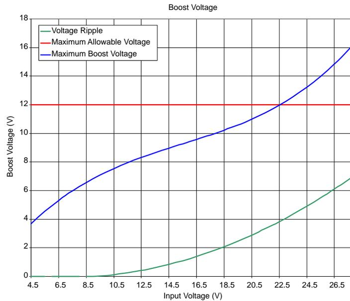
Figure 30. Boost Voltage at 80% Duty Cycle
