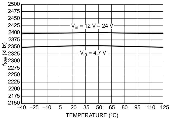
Figure 11. Switching Frequency vs Input Voltage and Temperature
