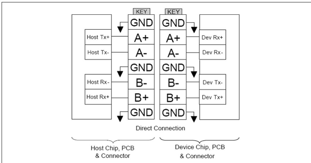
Figure 3-2 Direct Connection between the Host and Device
