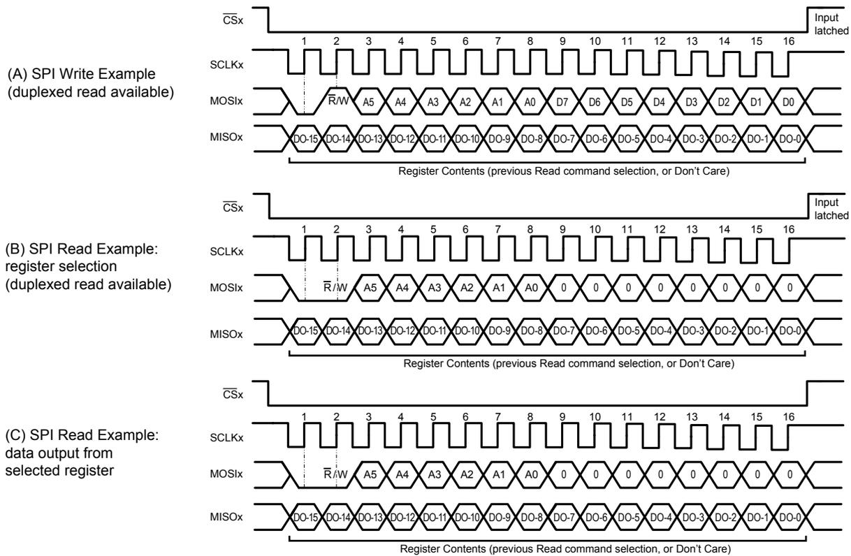
**Figure 28: SPI Read and Write Pulse Sequences**
