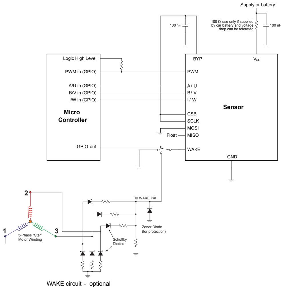
**Figure 41: Typical ABI / UVW Application Diagram**
