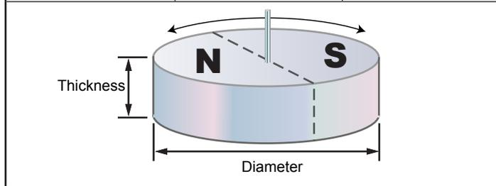
\* A sintered Neodymium magnet with 10 mm (or greater) diameter and 2.5 mm thickness is the recommended magnet for redundant applications.
