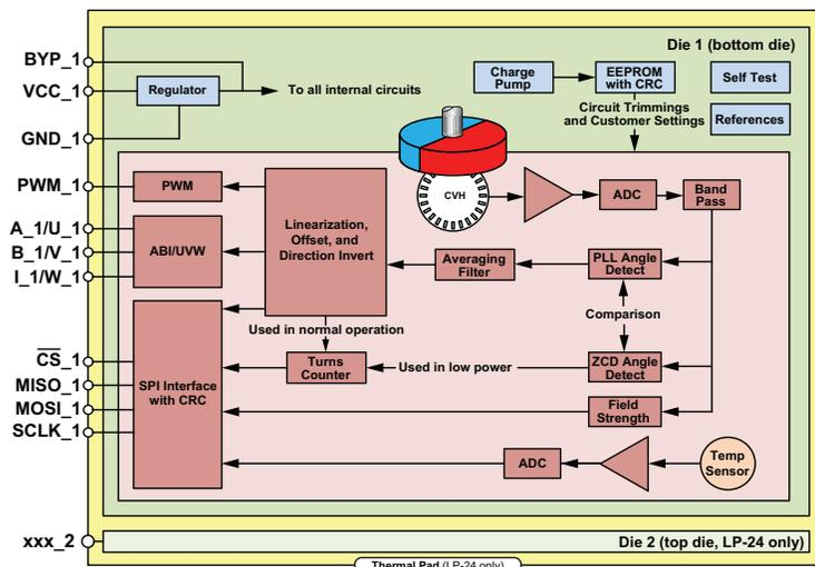
**Figure 1: AAS33051 Magnetic Circuit and IC Diagram**
