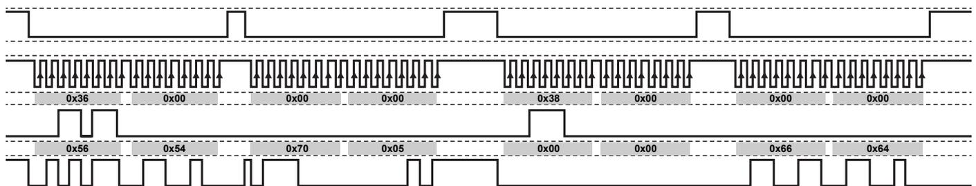
**Figure 17: Reading turns\_delta**
