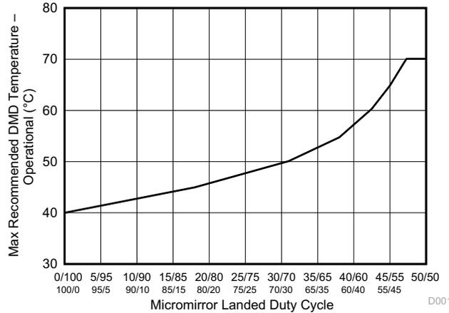
**Figure 7-1. Maximum Recommended DMD Temperature – Derating Curve**
