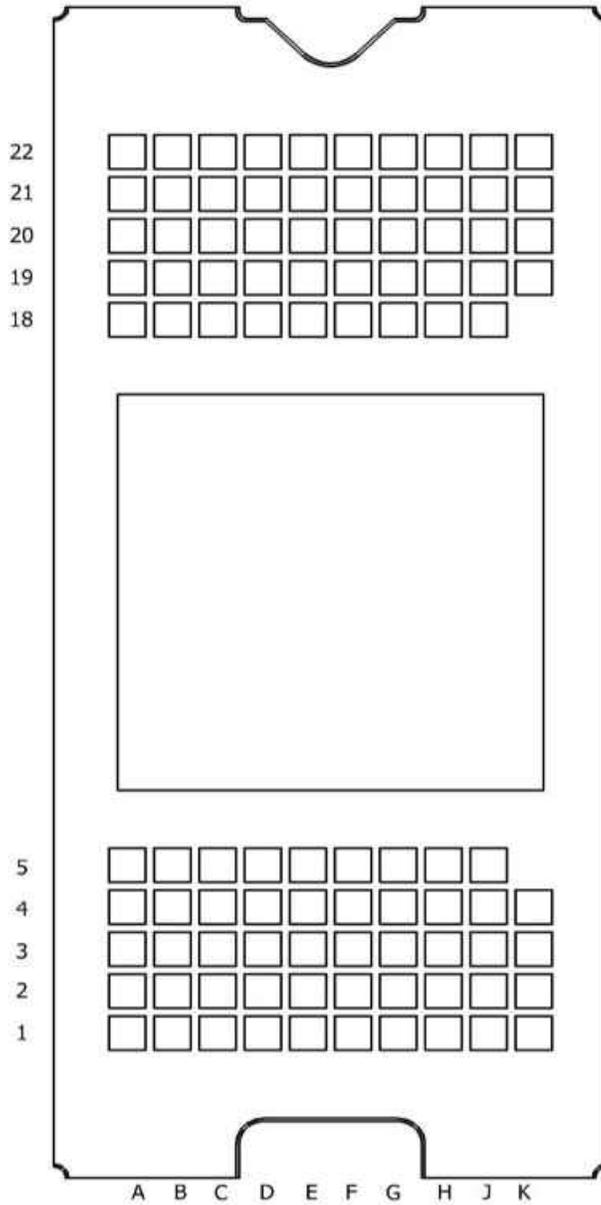
**Figure 6-2. FQD Package LCCC (98) Bottom View**
