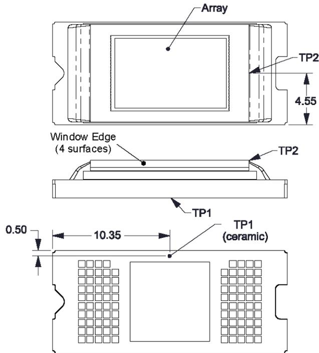
**Figure 8-4. Thermal Test Point Location - FQD Package**
