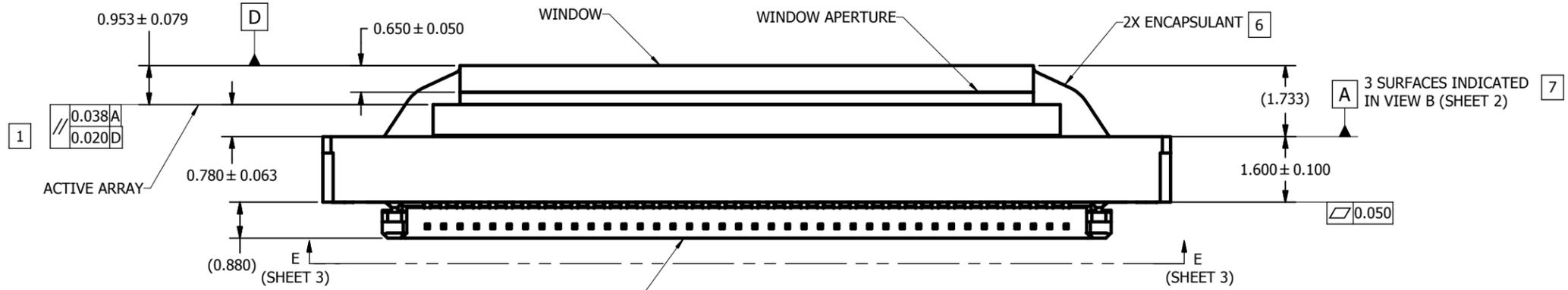
(PANASONIC AXT680124DD1, 80-CONTACT 0.4 mm PITCH BOARD-TO-BOARD CONNECTOR HEADER) MATES WITH PANASONIC AXT580124DD1 OR EQUIVALENT CONNECTOR SOCKET
