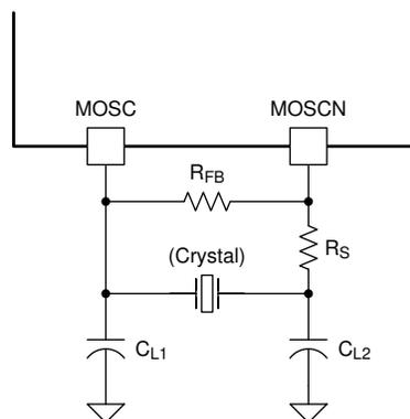
$C_L$  = crystal load capacitance in F
