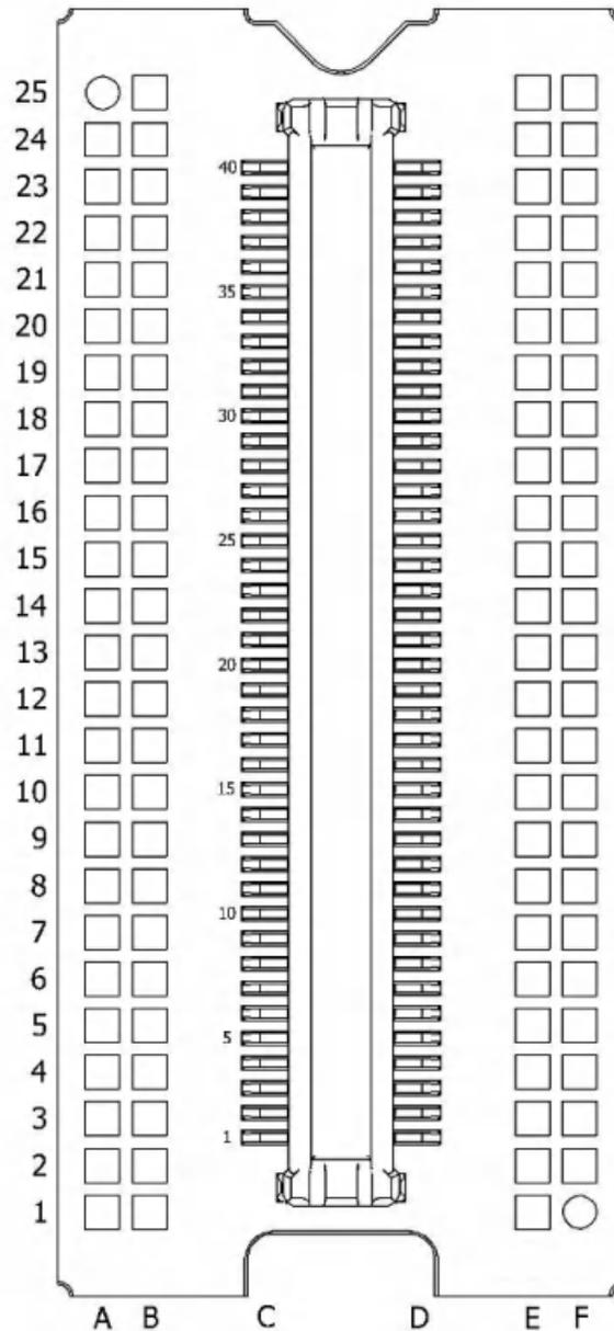
Figure 6-1. FQE Package. LCCC (80). Bottom View.
