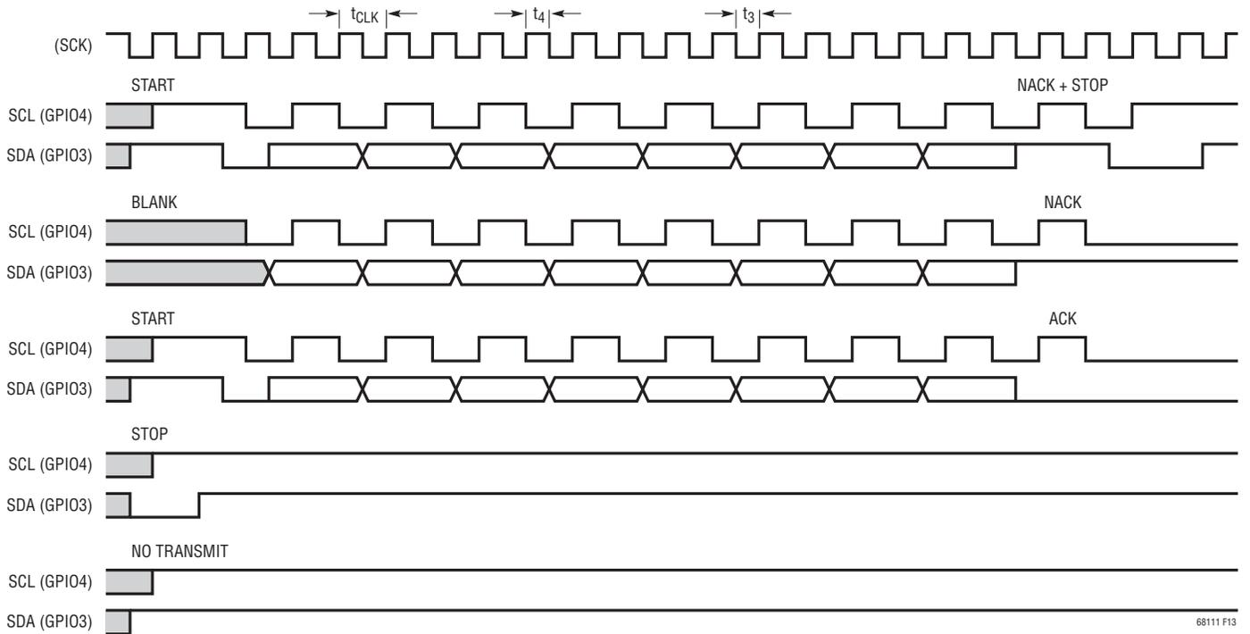
Figure 19. STCOMM Timing Diagram for an I<sup>2</sup>C Master
