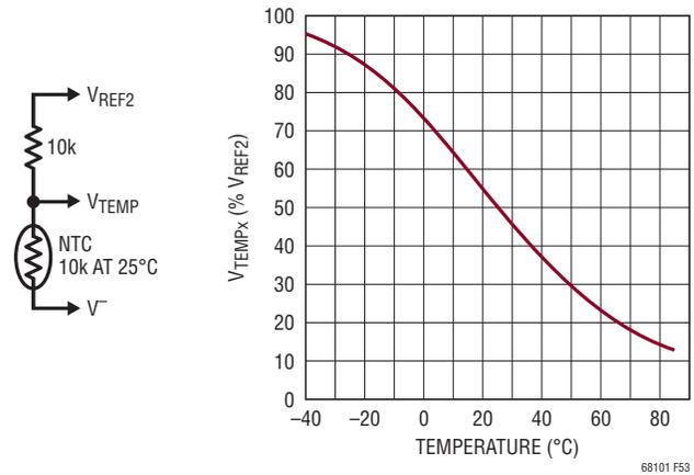
Figure 53. Typical Temperature Probe Circuit and Relative Output
