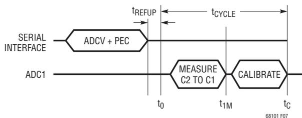
Figure 7. Timing for ADCV command measuring 1 cell, SCONV = 0
