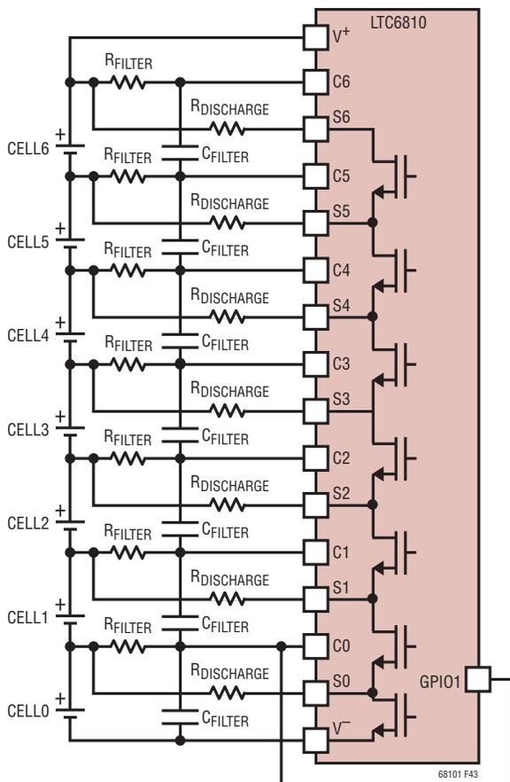
Figure 42. Seven Cell with Internal Discharge
