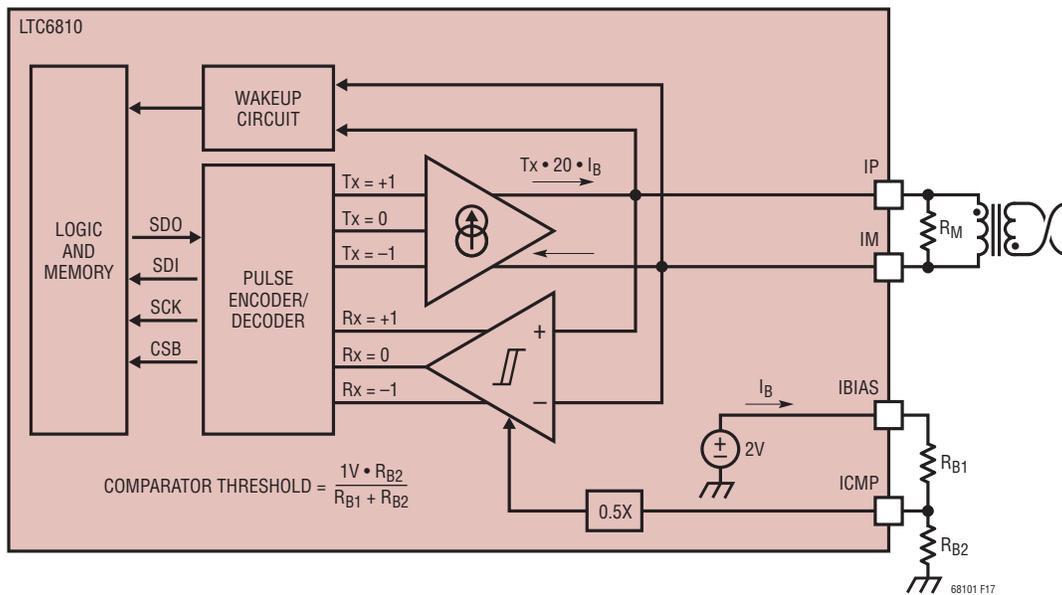
Figure 23. isoSPI Interface
