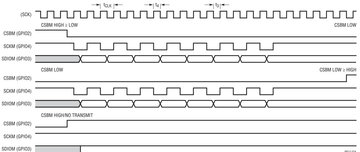
Figure 20. STCOMM Timing Diagram for a SPI Master
