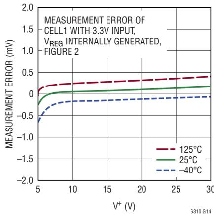
**Top Cell Measurement Error vs  $V^+$**
