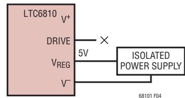
Figure 4.  $V_{REG}$  Powered by an Independent Supply
