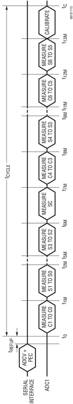
Figure 15. Timing of ADCVSC command, SCONV = 1
