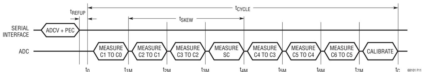
Figure 11. Timing for ADCVSC Command,  $SCONV = 0$
