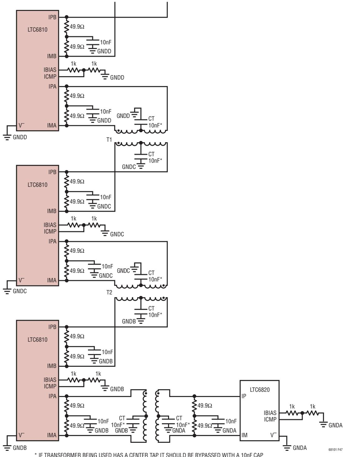
Figure 47. Daisy Chain Interface Components on Single Board
