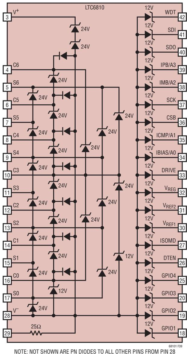
Figure 38. Internal ESD Protection Structures of the LTC6810
