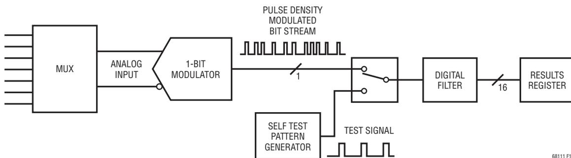
Figure 16. Operation of LTC6810 ADC Self Test
