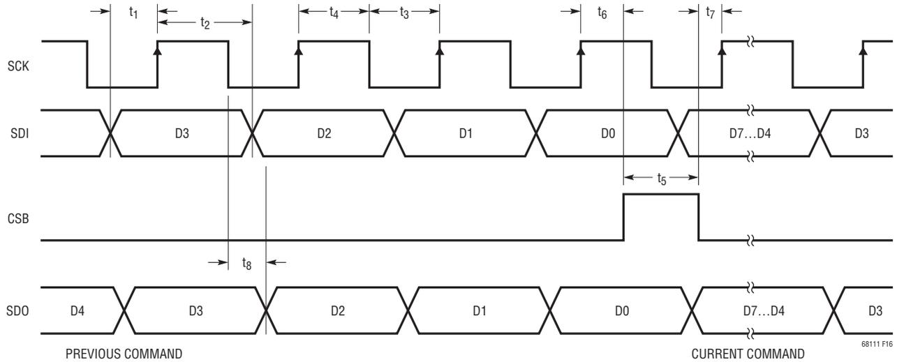
Figure 22. Timing Diagram of 4-Wire Serial Peripheral Interface
