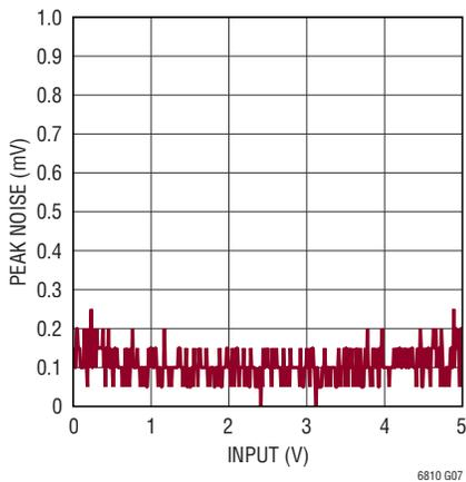
**Measurement Noise vs Input Filtered Mode**
