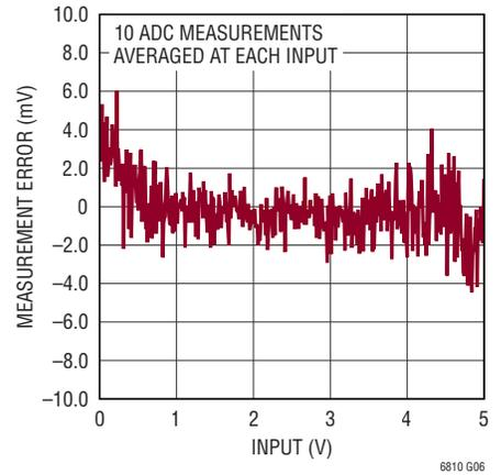
**Measurement Noise vs Input Normal Mode**
