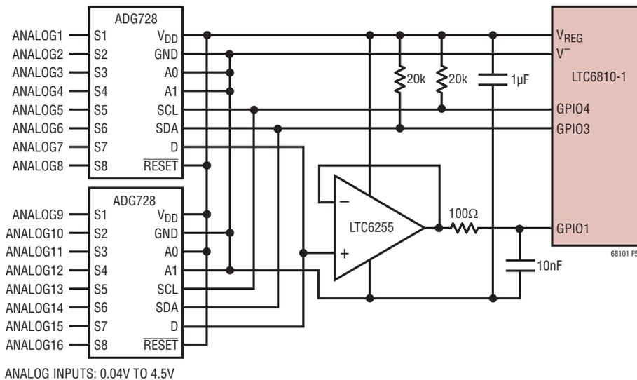
Figure 54. MUX Circuit Supports Sixteen Additional Analog Measurements
