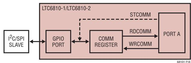
**Figure 18. LTC6810 I<sup>2</sup>C/SPI Master using GPIOs**
