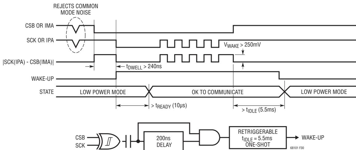
Figure 30. Wake-up Detection and IDLE Timer
