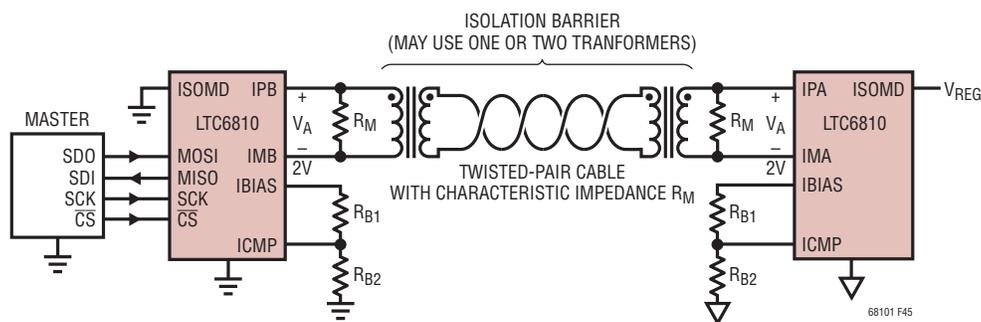
Figure 44. isoSPI Circuit
