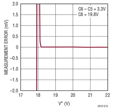
**Measurement Error vs Common Mode Voltage**
