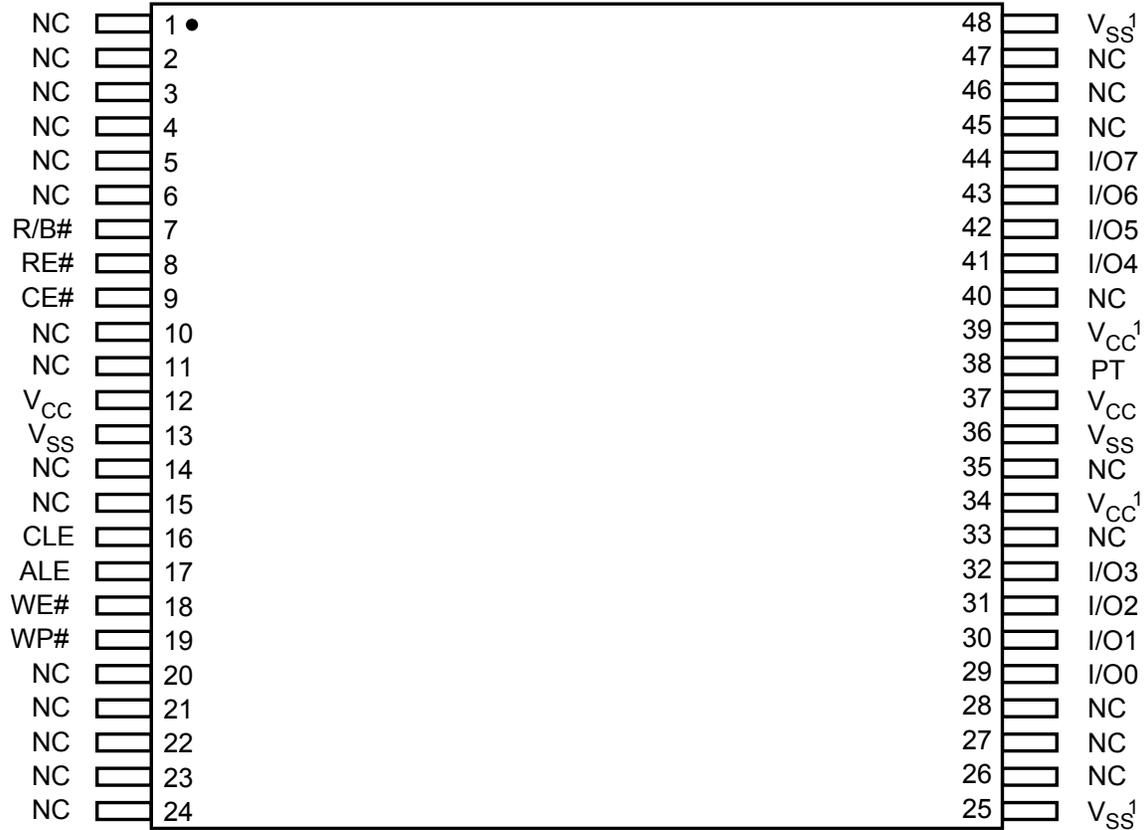
**Note 1.** These pins might not be connected internally. However, it is recommended to connect these pins to power(or ground) as designated for ONFI compatibility.
