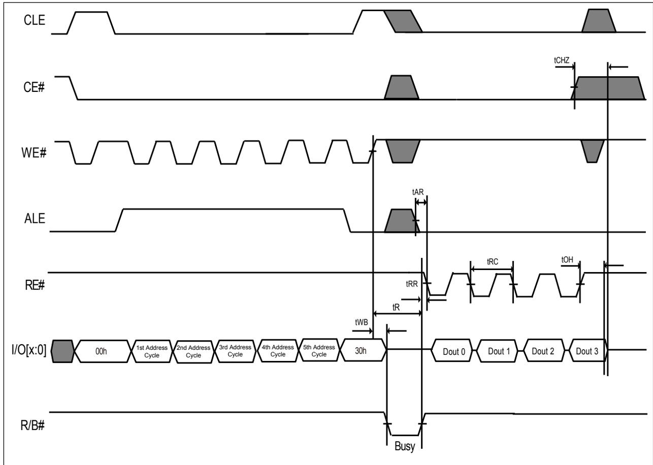
Figure 8. AC Waveforms for Read Operation (with CE# Don't Care)
