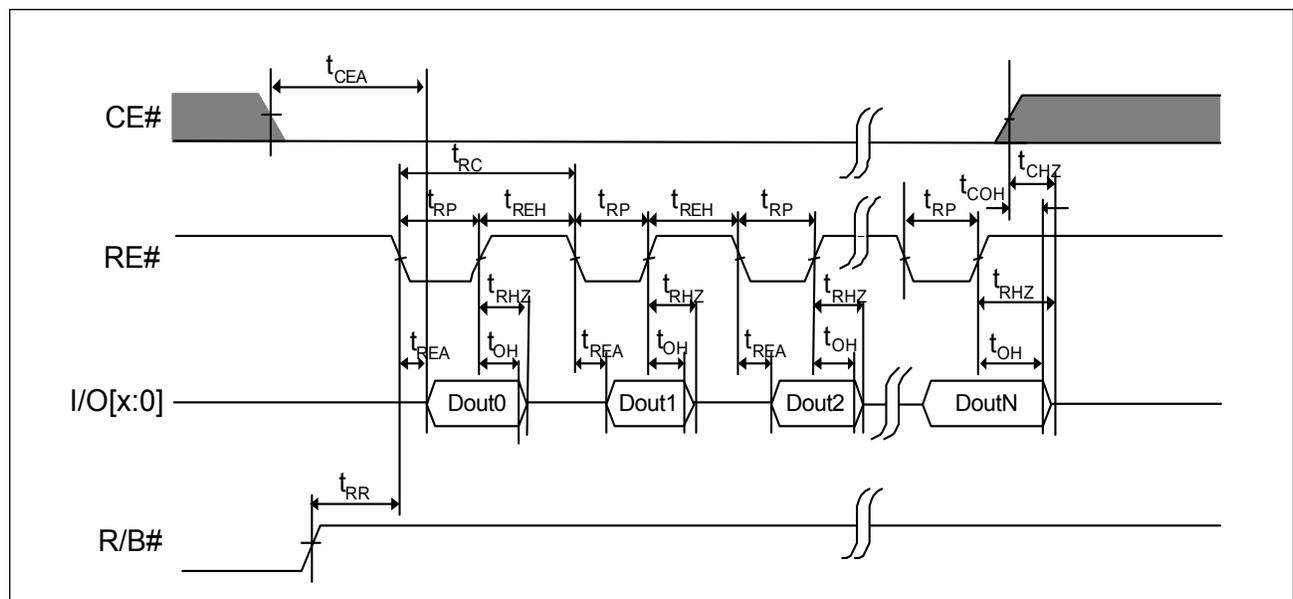
Figure 9-2. AC Waveforms for Sequential Data Out Cycle (After Read) - EDO Mode
