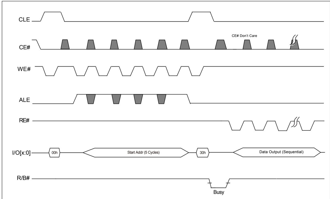
**Note:** The CE# "Don't Care" feature may simplify the system interface, which allows controller to directly download the code from flash device, and the CE# transitions will not stop the read operation during the latency time.
