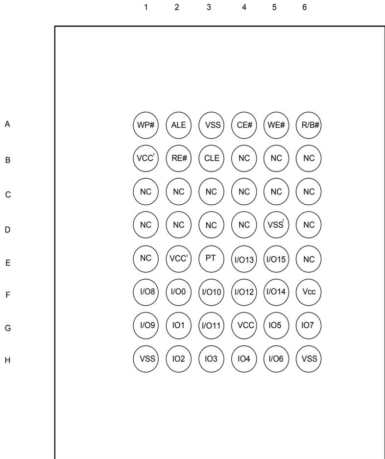
**Note 1.** *These pins might not be connected internally; however, it is recommended to connect these pins to power (or ground) as designated for ONFI compatibility.*
