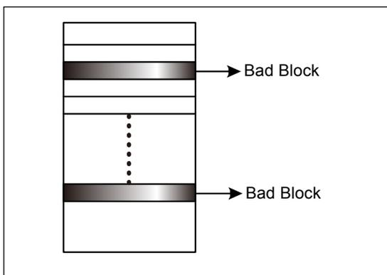
While the device is shipped, the value of all data bytes of the good blocks are FFh. The 1st byte of the 1st and 2nd page in the spare area for bad block will be 00h for x8; and 0000h for x16. The erase operation at the bad blocks is not recommended.
