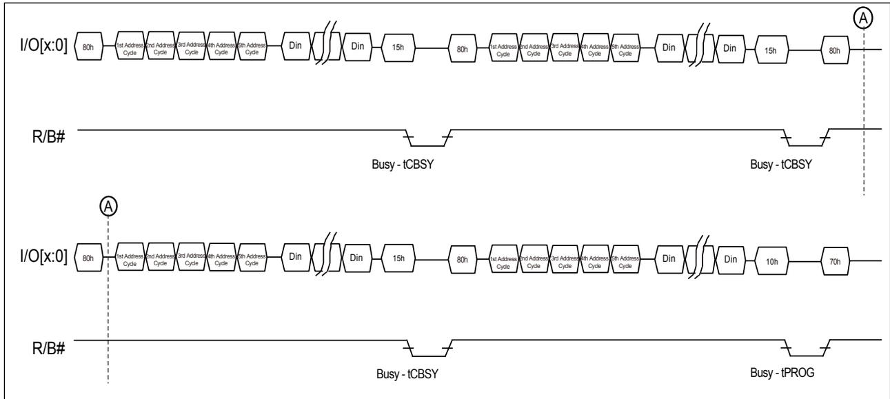
**Note:**  $tPROG = Page_{(Last)} \text{ programming time} + Page_{(Last-1)} \text{ programming time} - \text{Input cycle time of command \& address} - \text{Data loading time of page}_{(Last)}$ .
