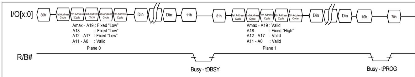
**Figure 39. AC waveforms for Two-plane Cache Program (Traditional)**
