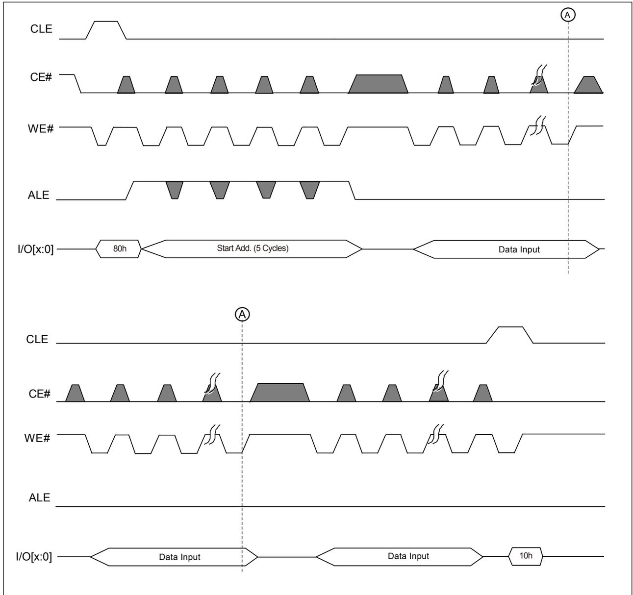
**Note:** The CE# "Don't Care" feature may simplify the system interface, which allows the controller to directly write data into flash device, and the CE# transitions will not stop the program operation during the latency time.
