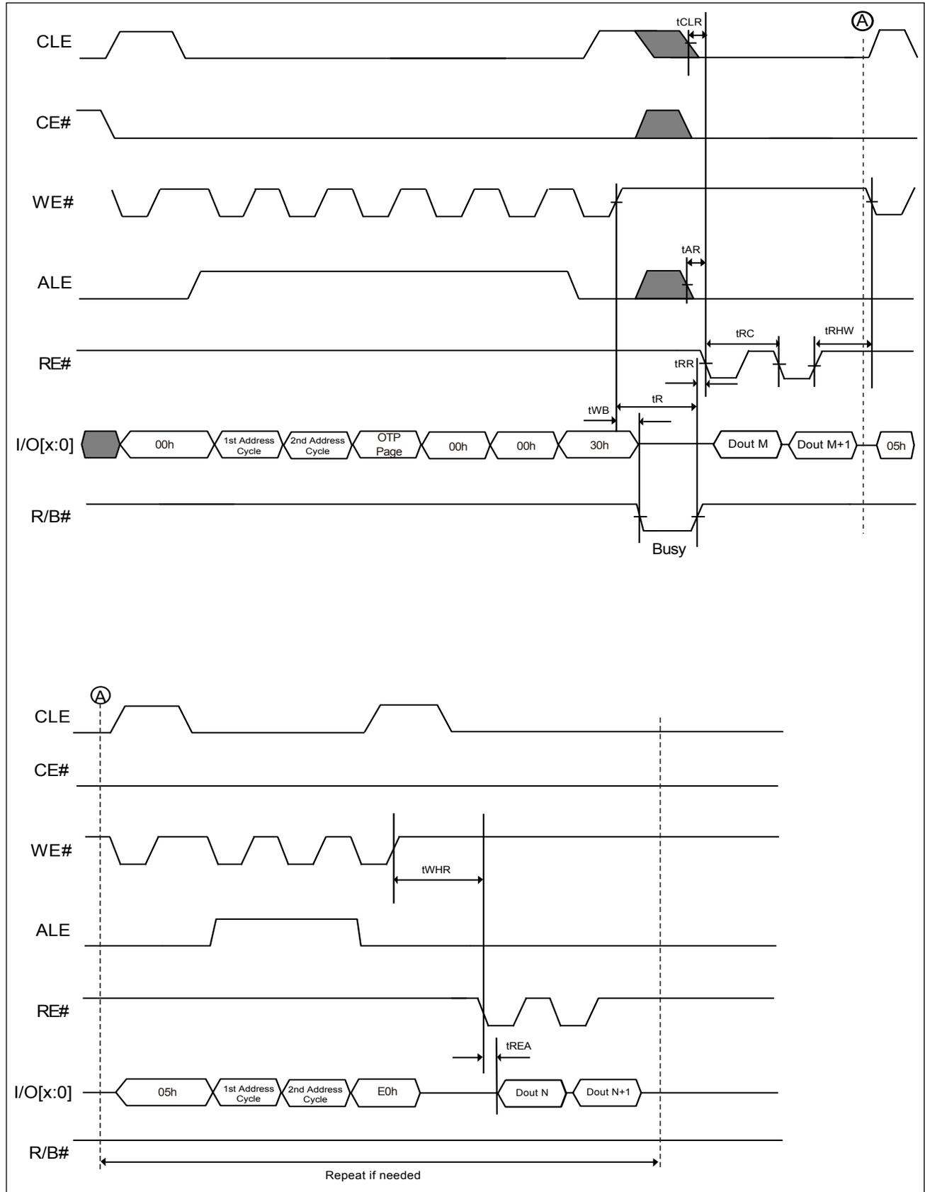
Figure 31. AC Waveforms for OTP Data Program
