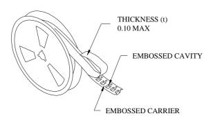
• THE FORCE FOR TEARING OFF COVER TAPE IS 10 TO 100 GRAMS IN THE ARROW DIRECTION.
