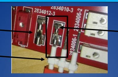
Wire stops prevent the pins from traveling past the end of the contact to absorb mating tolerances in both contacts and connectors
