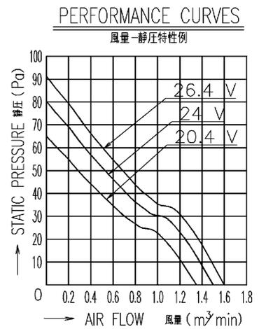
NOTE: 1. MEASURED AT 1 m DISTANCE FROM THE AIR INLET.
