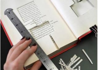
The coil should be as close to the cover as possible, but you might want to make the spot for the circuit a bit deeper so the USB connector is completely submerged in pages.
