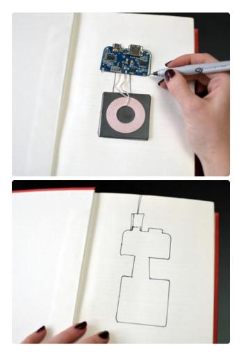
Open the front cover and place the transmitter on the first page. Trace around the outline and set the transmitter aside.
