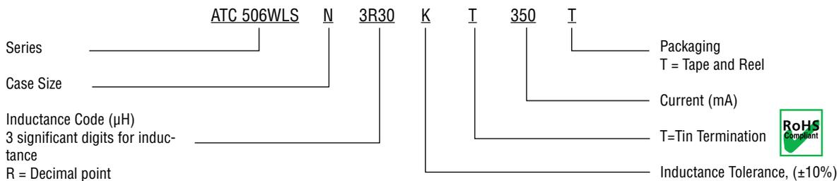
The above part number refers to a 506WLS Series, Case Size N, 3.30 μH inductor, K tolerance (±10%, typ.), with Tin Termination (T), 350 mA, tape and reel packaging.
