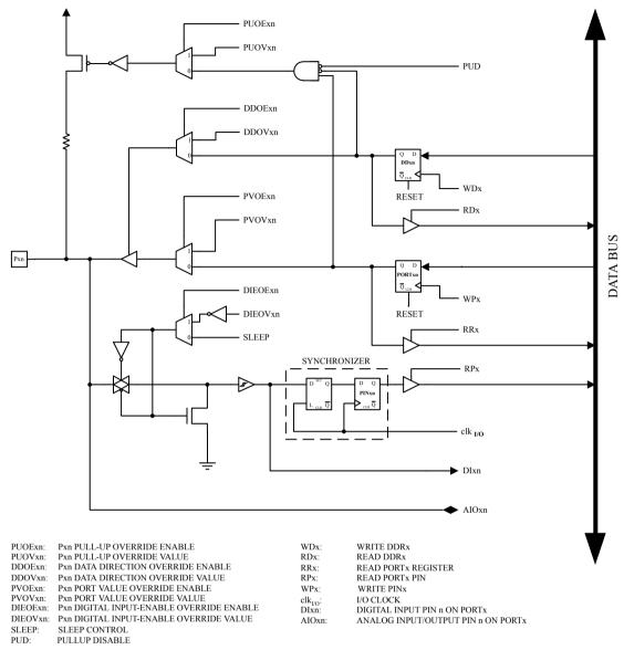
**Note:** 1. WPx, WDx, RRx, RPx, and RDx are common to all pins within the same port.  $clk_{I/O}$ , SLEEP, and PUD are common to all ports. All other signals are unique for each pin.
