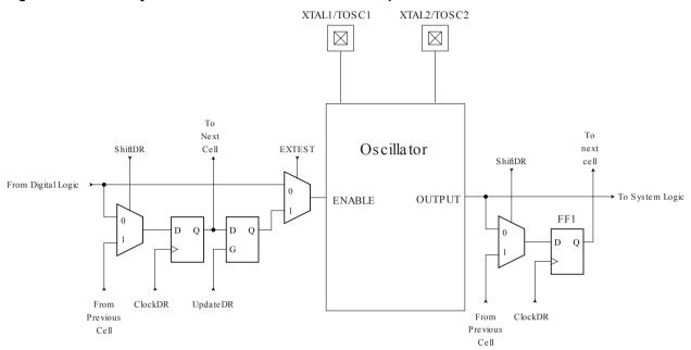
The following table summaries the scan registers for the external clock pin XTAL1, oscillators with XTAL1/XTAL2 connections as well as 32kHz Timer Oscillator.
