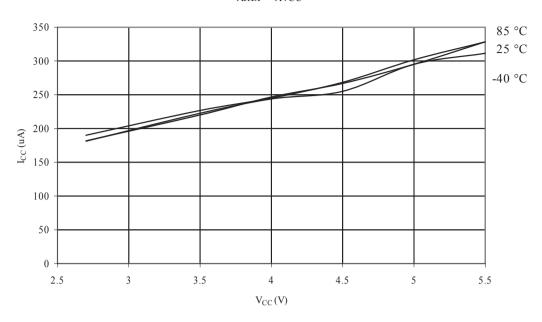
Figure 31-49. AREF External Reference Current vs. V<sub>CC</sub>
