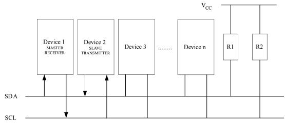
A START condition is sent by writing to the TWI Control register (TWCR) a value of the type TWCR=1x10x10x:
