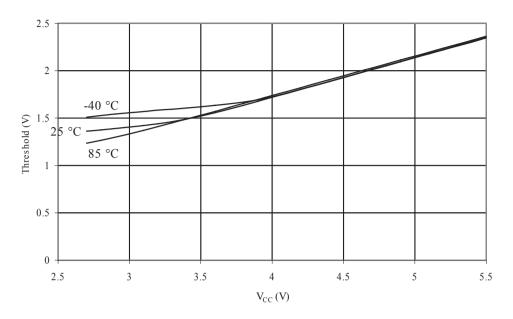
Figure 31-29. Reset Input Threshold Voltage vs. V<sub>CC</sub> (V<sub>IL</sub>,Reset Pin Read as "0")
