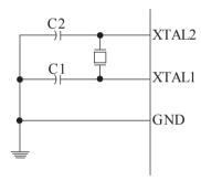
The Oscillator can operate in three different modes, each optimized for a specific frequency range. The operating mode is selected by the fuses CKSEL3:1 as shown in the following table.
