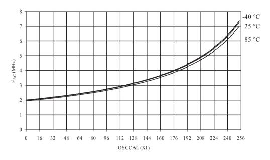
Figure 31-41. Calibrated 2MHz RC Oscillator Frequency vs. Temperature
