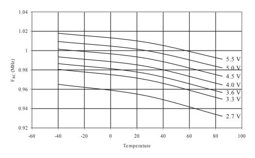
Figure 31-45. Calibrated 1MHz RC Oscillator Frequency vs.  $V_{\text{CC}}$
