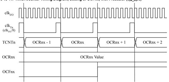
Figure 19-11. Timer/Counter Timing Diagram, Setting of OCFnx, with Prescaler (fclk 1/0/8)
