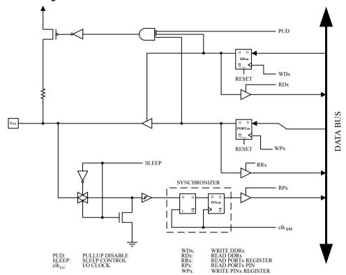
**Note:** 1. WPx, WDx, RRx, RPx, and RDx are common to all pins within the same port.  $clk_{I/O}$ , SLEEP, and PUD are common to all ports
