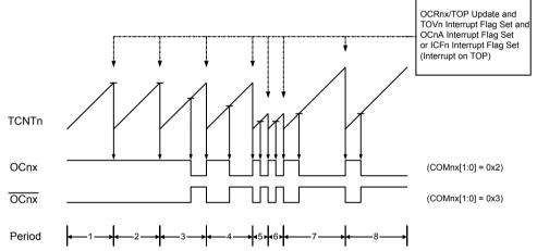
The Timer/Counter Overflow Flag (TOVn) is set each time the counter reaches TOP. In addition the OCFnA or ICFn Flag is set at the same timer clock cycle as TOVn is set when either OCRnA or ICRn is used for defining the TOP value. If one of the interrupts are enabled, the interrupt handler routine can be used for updating the TOP and compare values.
