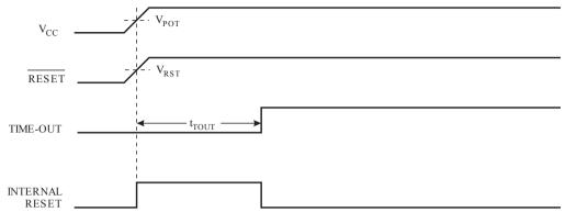
Figure 14-3. Figure: MCU Start-up, RESET Extended Externally
