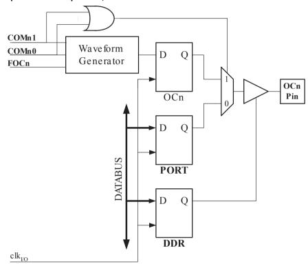
The general I/O port function is overridden by the Output Compare (OC0) from the waveform generator if either of the COM01:0 bits are set. However, the OC0 pin direction (input or output) is still controlled by the Data Direction Register (DDR) for the port pin. The Data Direction Register bit for the OC0 pin (DDR\_OC0) must be set as output before the OC0 value is visible on the pin. The port override function is independent of the Waveform Generation mode.
