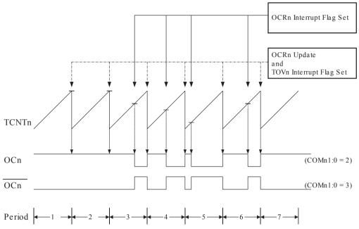
The Timer/Counter Overflow Flag (TOV0) is set each time the counter reaches MAX. If the interrupt is enabled, the interrupt handler routine can be used for updating the compare value.
