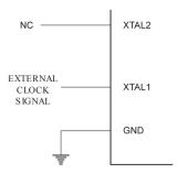
When this clock source is selected, start-up times are determined by the SUT Fuses as shown in the following table.
