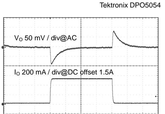
Figure 17. Load Response 1 ( $V_{IN} = 13.2\text{ V}$ ,  $I_O = 1.5\text{ A} \rightarrow 2.0\text{ A}$ ,  $200\ \mu\text{s} / \text{div}$ )
