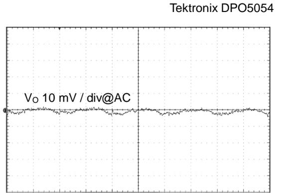
Figure 15. Output Ripple Voltage 1 ( $V_{IN} = 13.2\text{ V}$ ,  $I_O = 1.5\text{ A}$ ,  $1\ \mu\text{s} / \text{div}$ )
