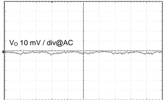
Figure 19. Output Ripple Voltage 2
