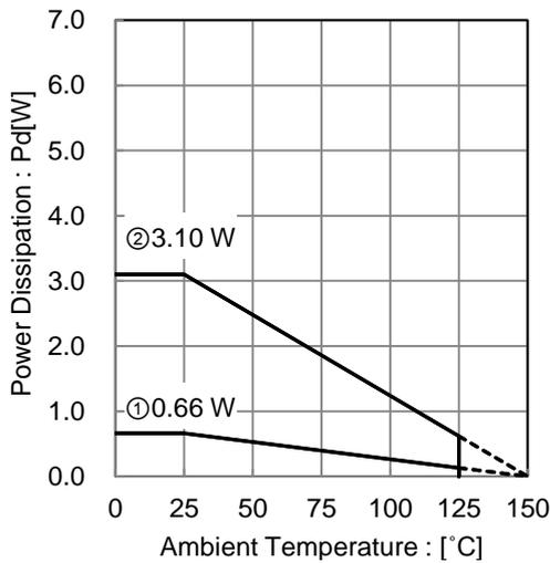
① IC mounted on ROHM standard board based on JEDEC51-3
