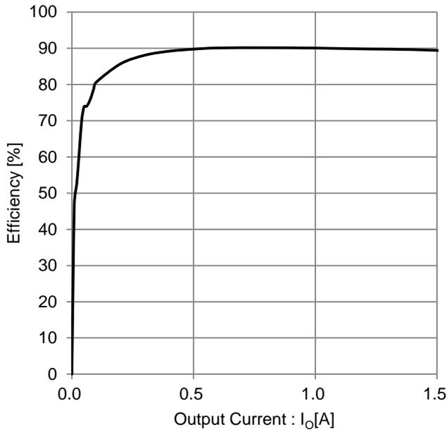
Figure 18. Efficiency vs Output Current
