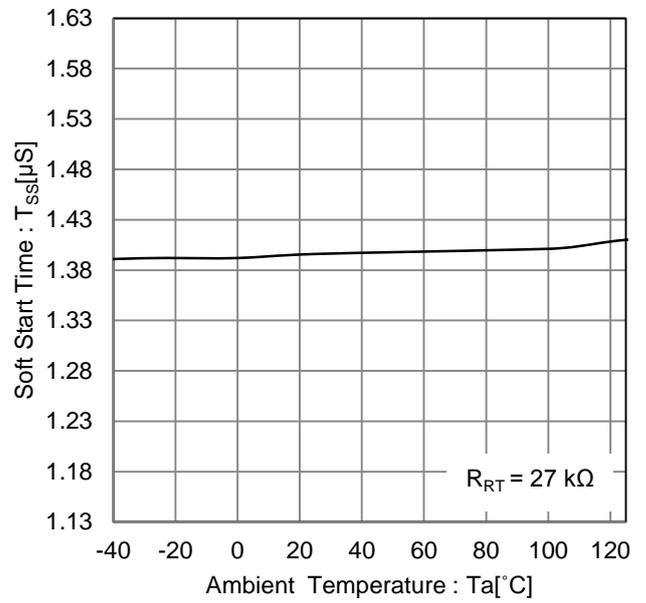
Figure 8. Soft Start Time vs Ambient Temperature
