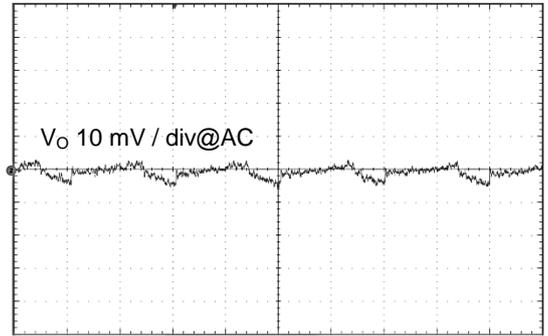
Figure 31. Output Ripple Voltage 5
