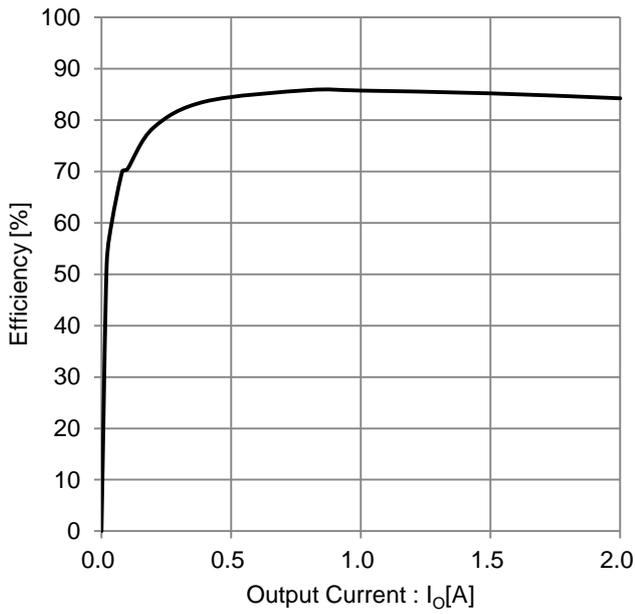
Figure 26. Efficiency vs Output Current
