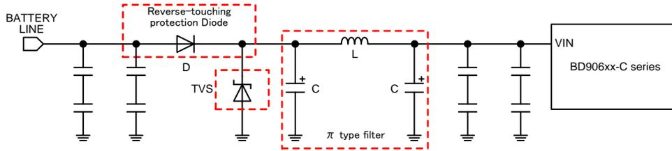
Figure 34. Filter Circuit
