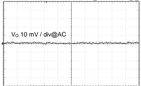
Figure 23. Output Ripple Voltage 3
