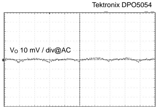
Figure 27. Output Ripple Voltage 4
