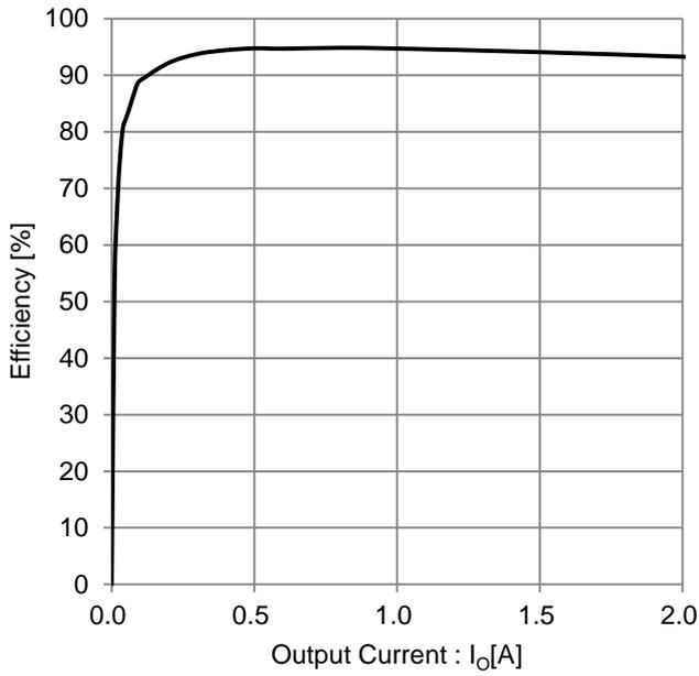
Figure 30. Efficiency vs Output Current
