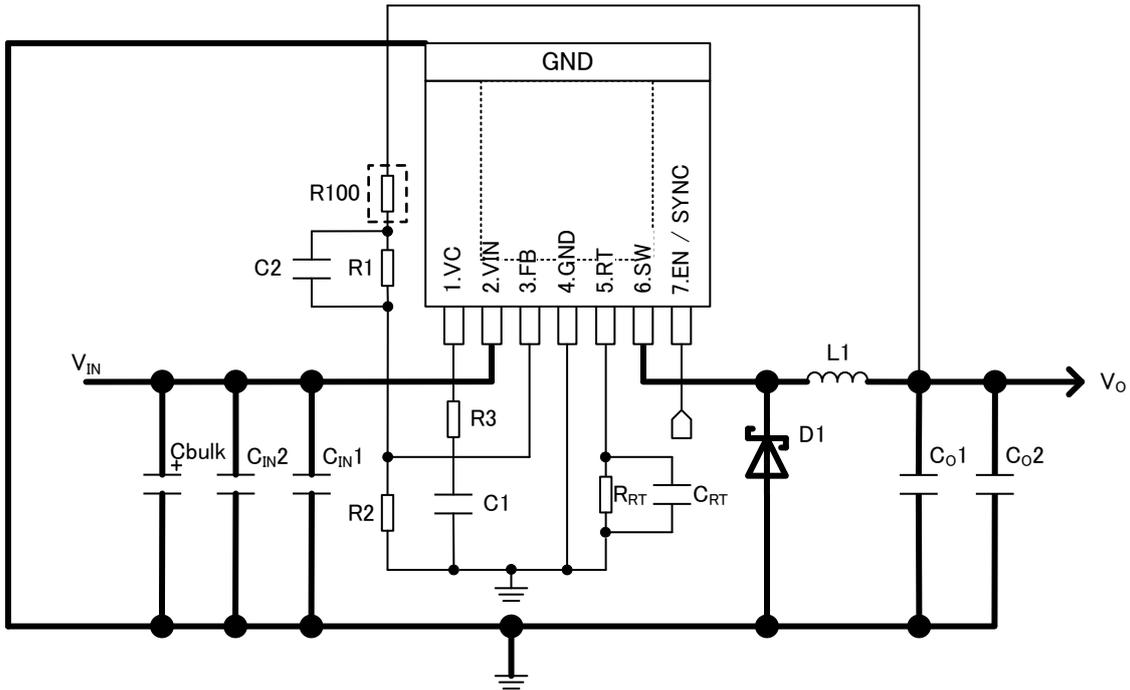
Exposed die pad is needed to be connected to GND.
