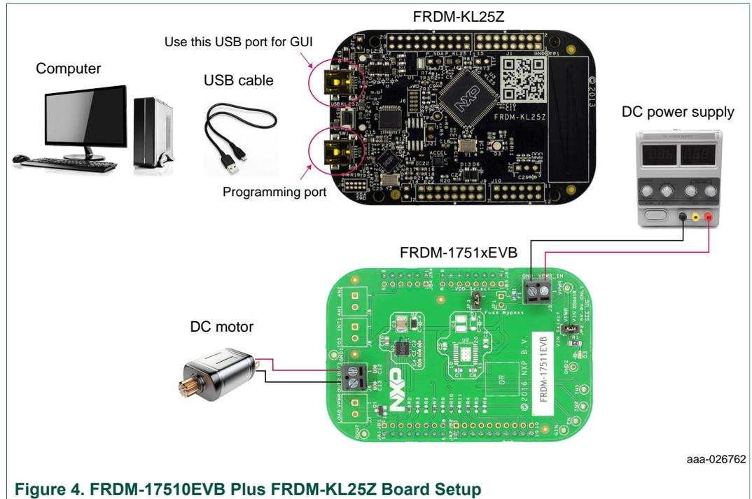
Figure 4. FRDM-17510EVB Plus FRDM-KL25Z Board Setup
