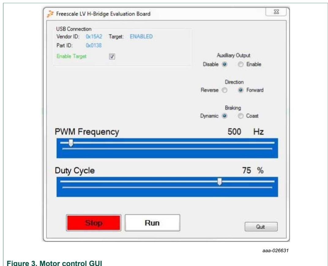
Figure 3. Motor control GUI
