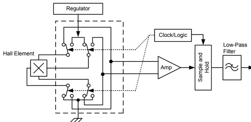
Figure 3: Chopper Stabilization Circuit (Dynamic Quadrature Offset Cancellation)
