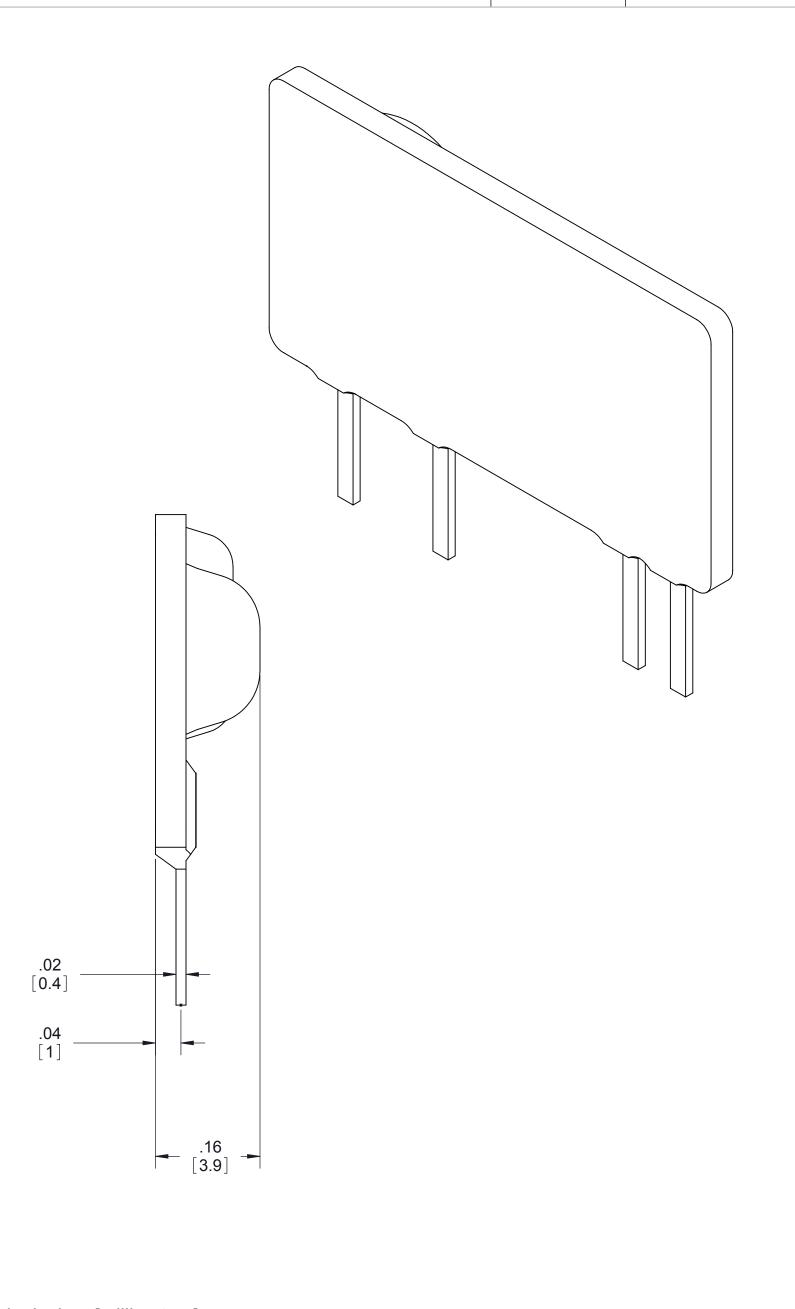
Tolerances: ± 0.02 in / 0.5 mm. All dimensions are in: inches [millimeters]
