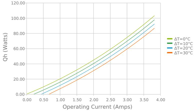
Total Heat Dissipated at Hot Side (Qh=Qc+Pin)
