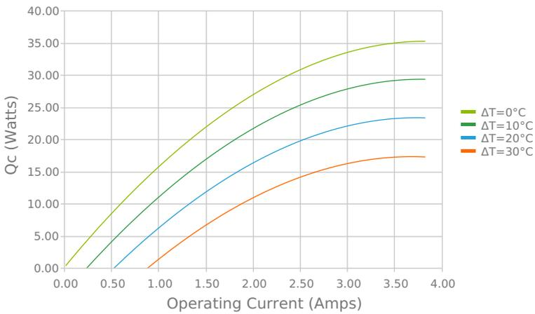
Heat Pumped at Cold Side ( $Q_c$ )
