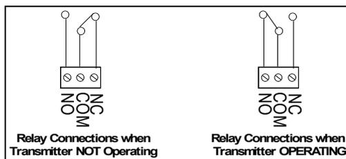
The action of the relay outputs is set by Option link setting Jumper. A link is made / removed by the small shorting link 'cap' placed over the pin header.
