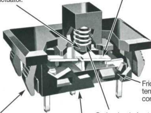
Friction fit of terminals keeps contaminants out.
