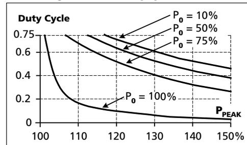
$$\text{DutyCycle} = \frac{T_{\text{peak}}}{T_{\text{peak}} + T_0}$$
