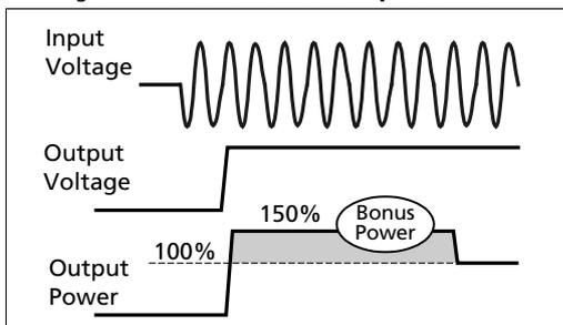
Fig. 6-8 BonusPower<sup>®</sup> after output short
