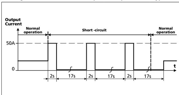
Fig. 6-4 Dynamic overcurrent capability, typ.
