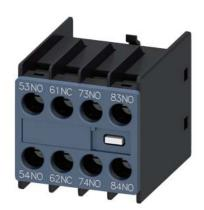
Auxiliary switch on the front, 3 NO + 1 NC Current path 1 NO, 1 NC, 1 NO, 1 NO for 3RH and 3RT screw terminal 53/54, 61/62, 71374, 83/84
