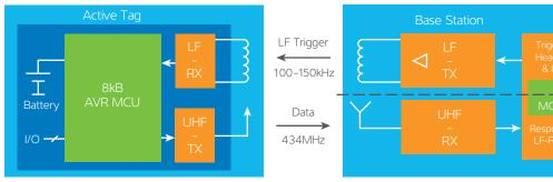
\*1) Graph shows one combined base station. Option is to split that as RX distance is much higher. So multiple trigger stations and one or few RX stations.
