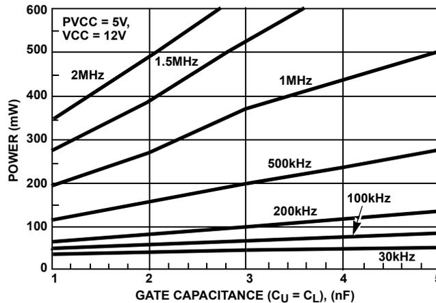
FIGURE 8. POWER DISSIPATION vs LOADING, PVCC = 5V
