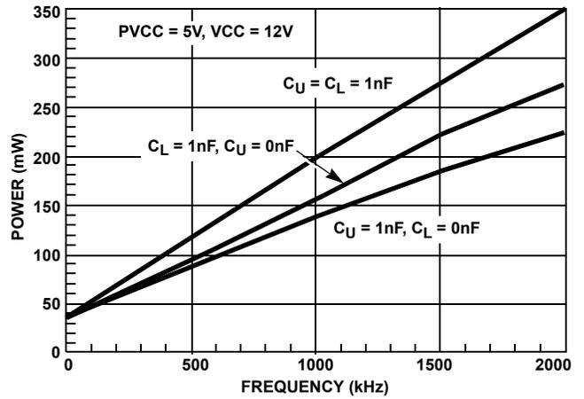
FIGURE 7. POWER DISSIPATION vs FREQUENCY, PVCC = 5V
