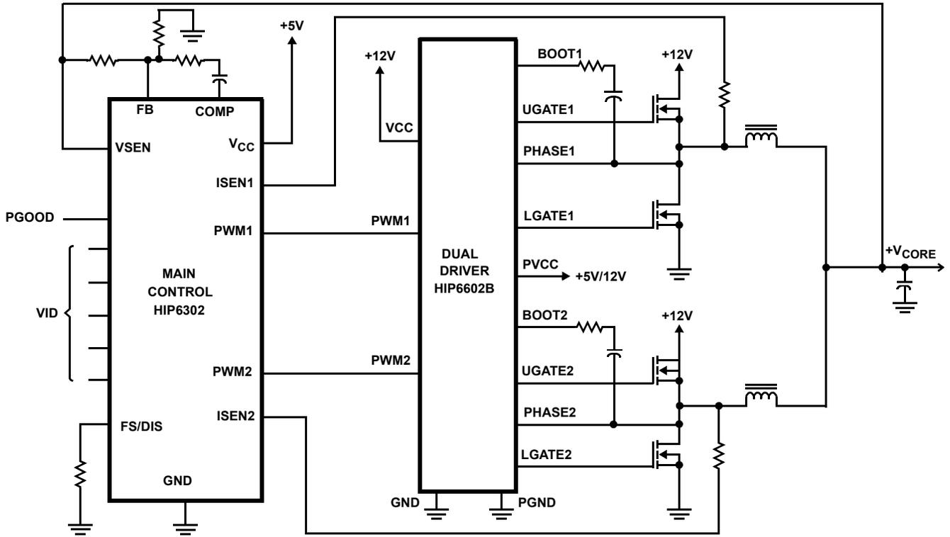
Typical Application - 4 Channel Converter Using a HIP6303 and HIP6602B Gate Driver
