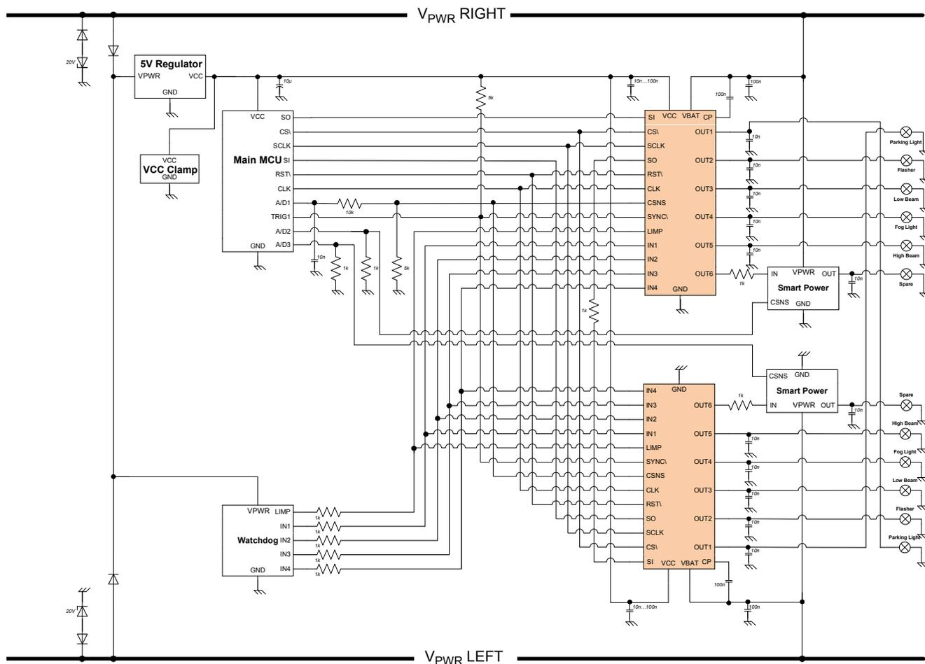
Figure 36. Typical Front Lighting Application for Automotive
