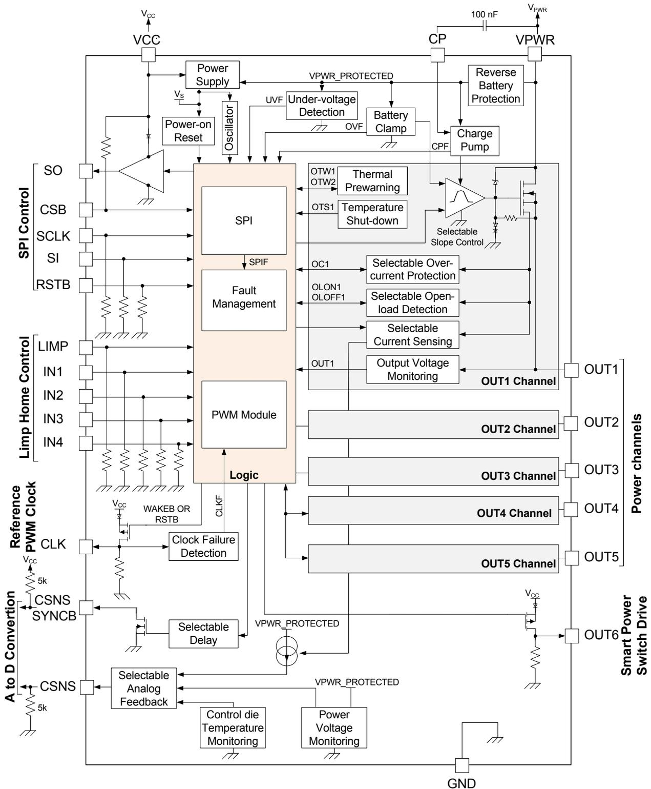
Figure 2. Simplified Internal Block Diagram (Penta version)
