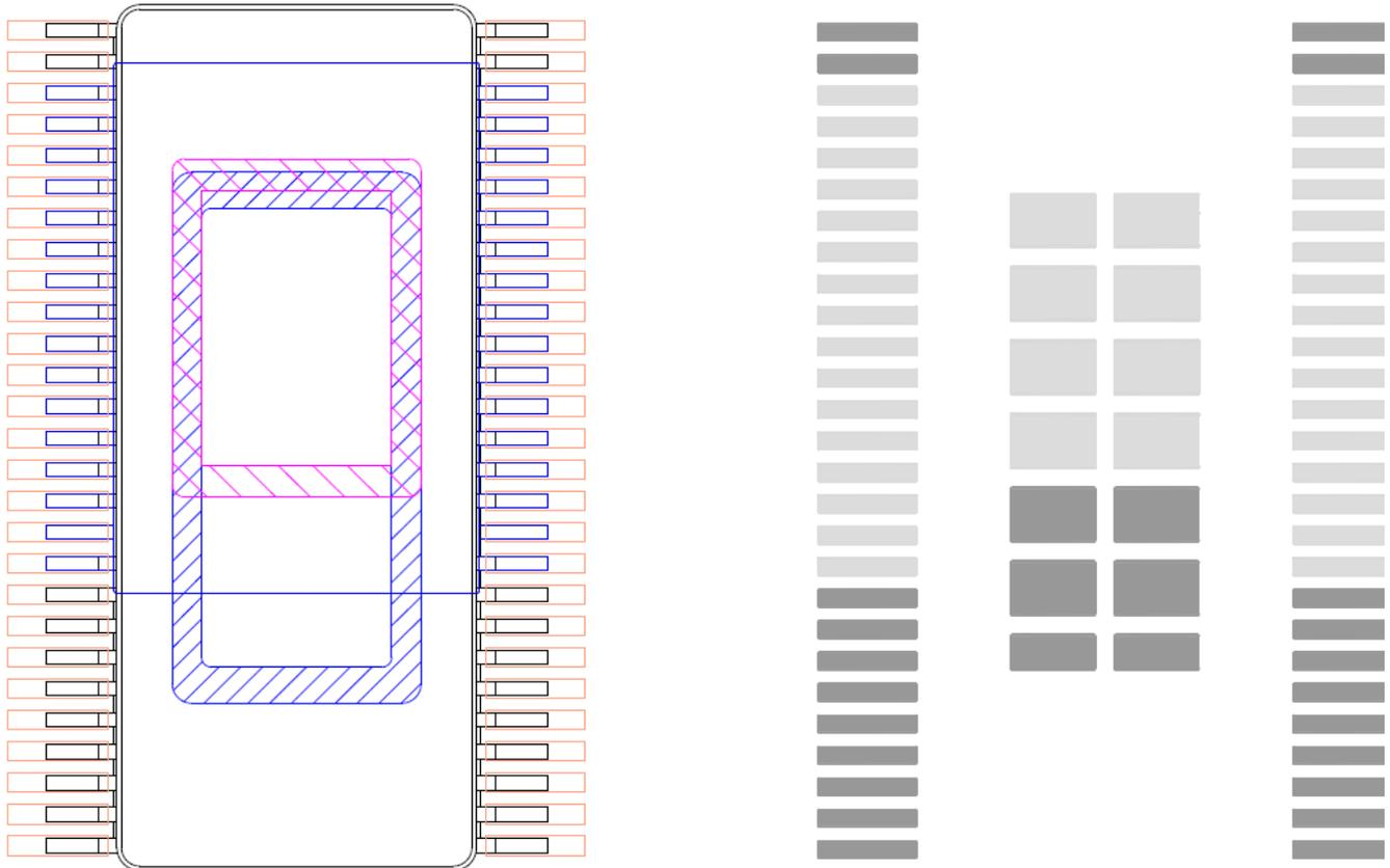
Figure 37. PCB Copper Layer & Solder Stencil Opening Recommendations
