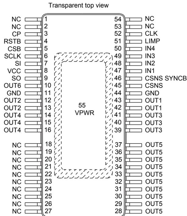
Figure 3. Pinout Diagram
