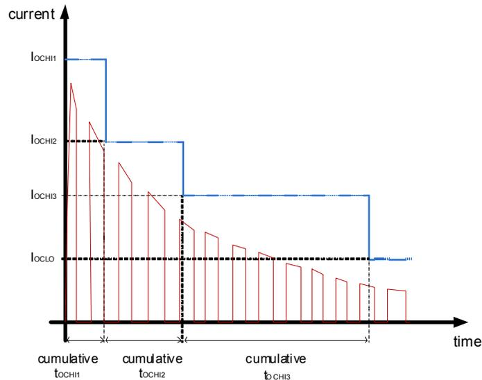
**Figure 16. Transient Over Current Profile in PWM mode**
