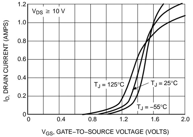
Figure 2. Transfer Characteristics
