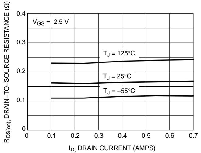
Figure 4. On-Resistance vs. Drain Current and Temperature
