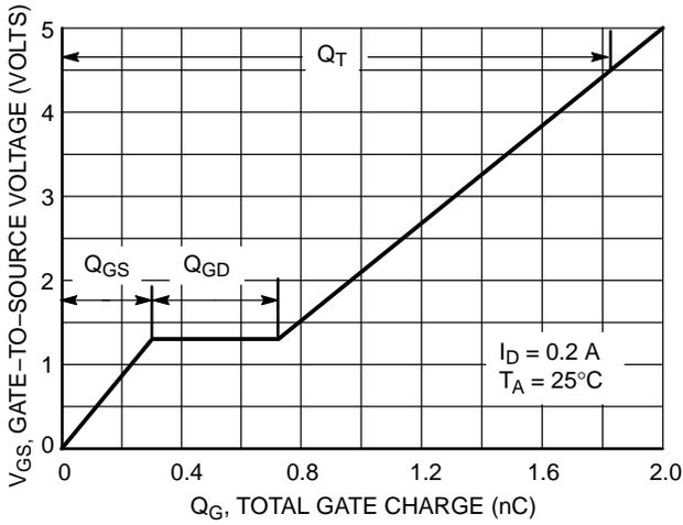
Figure 7. Gate-to-Source Voltage vs. Total Gate Charge
