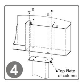
Attach the RS001-0223 Respiratory Hygiene Station to the column using (4x) screws included with stand. Tighten.
