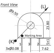
All dimensions are in mm Linear dimensional tolerance ±0.2mm
